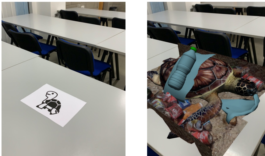
Figure 16. Screen capture of the AR experience during the focus group: process of marker recognition (left) and projection of a digital 3D object on the real world in real time (right)
