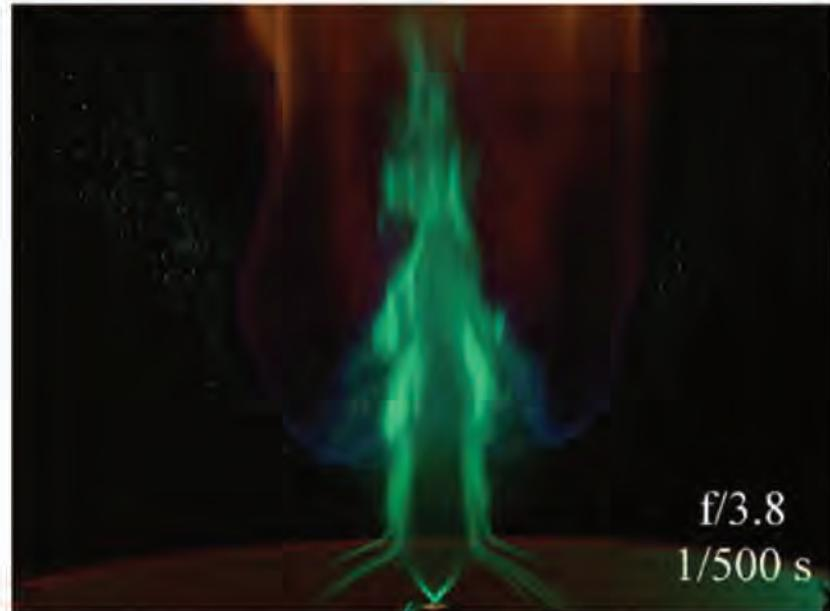
**Fig. 2.20.** Smoke visualization photographs of the experiment of Marley *et al.* [59]. The smoke is injected upstream of the nozzle on both sides of the burner (though emanating from different radii in the co-flow) to visualize air entrainment.
