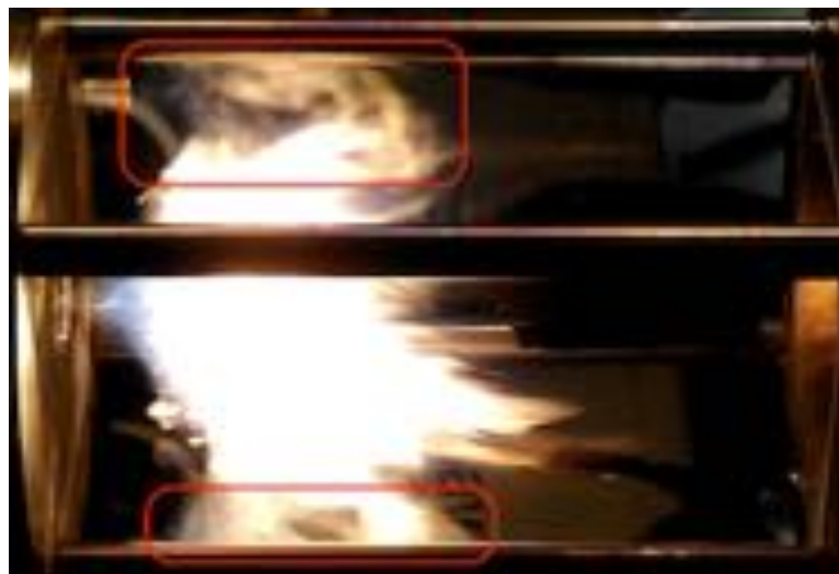
Figure 9.12: UTIAS configuration: Visualization of soot for the selected operating conditions. (Courtesy of Wang et al. )
