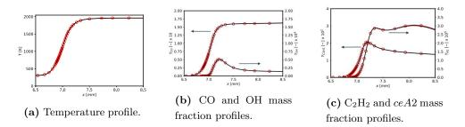
Figure 5.10: One-dimensional premixed unstrained ethylene-air laminar flame at P = 3 bars and equivalence ratio  $\phi = 2.0$ . Comparison between BISETTI (----), C2H4\_A2\_28\_205\_14\_LG (O). of T (a), CO and OH (b) and C<sub>2</sub>H<sub>2</sub> (c).
