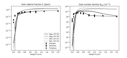
Figure 6.18: Effect of Bi-variate description on soot predictions. Comparison between numerical models and measurements.
