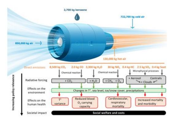
Figure 1.4: Emissions from a typical two-engine jet aircraft during 1-hour flight with 150 passengers (extracted from the *European Aviation Environmental Report 2019*), and their impact (adapted from the European Aviation Environmental Report 2019, *Masiol et al.* 3 and *Lee et al.* 4).
