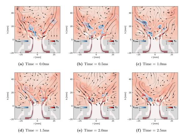
Figure 8.25: FIRST configuration: Sequence of mixture fraction Z with overlaid blue  $C_2H_2$  mass fraction, flow field velocity is represented by arrowed by streamlines with a width proportional to the local velocity intensity for the case RUN\_HL\_A4.
