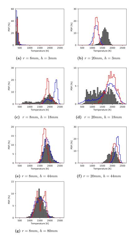
**Figure 8.9:** FIRST configuration: Probability Density Functions of temperature at various locations along the radial axis. Comparison between simulation with (red lines) and without (blue lines) thermal radiation, and CARS measurements (grey).
