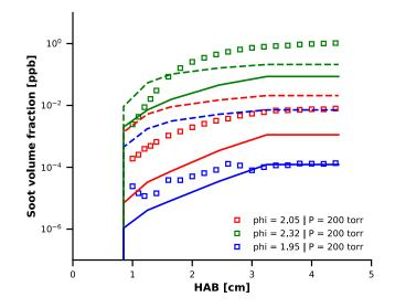
Figure 6.11: Soot prediction in nucleation flames. Comparison between experiments 285 and Lagrangian Soot Tracking with different soot precursors species.
