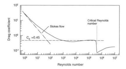
**Figure 3.7:** Drag coefficient  $\mathcal{C}_D$  as function of the particle Reynolds number  $Re_p$ . Extracted from Crowe et al [240].
