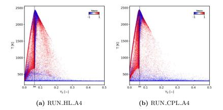
**Figure 8.15:** FIRST configuration: Scatterplots of temperature as a function of mixture fraction colored by the Takeno Index in the primary zone for cases RUN\_HL\_A4 (a) and RUN\_CPL\_A4 (b).
