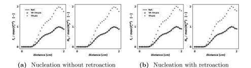
Figure 7.5: Comparison of predicted soot volume fraction (considering only nucleation) with and without soot model scaling in a rich premixed flame with constant thickening  $(\mathcal{F} = 2)$  and the resolved flame (without thickening).
