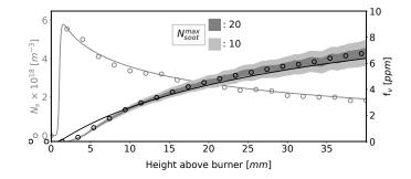
Figure 4.6: Soot number density (left) and soot volume fraction (right axis) for coagulation in the ISF Target Flame 4 (Laminar Premixed Pressurised 2). Comparison between EE (lines) and LST (symbols), shaded area indicate the stochastic noise of LST for two values of  $N_{soot}^{max}$ .
