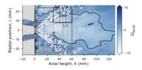
Figure 9.5: UTIAS configuration: Instantaneous axial velocity from LES in a mid-plane cut. Black line: isoline of zero-axial velocity to mark recirculate zones. The spray is superimposed in white via the liquid volume fraction.
