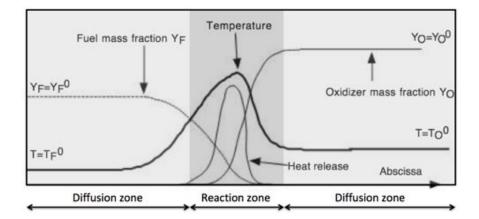
Figure 3.4: Laminar diffusion flame structure. Extracted from Poinsot & Veynante 197.
