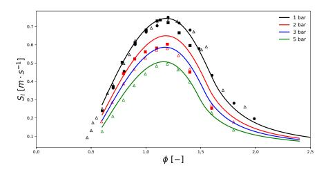
**Figure 5.6:** Flame speed of ethylene flames at various pressures: *Bisetti et al.* mechanism [231] (lines), *Hassan et al.* [276] ( $\blacksquare$ ), *Egolfopoulos et al.* [277] ( $\triangle$ ), *Jomaas et al.* [278] ( $\bullet$ )
