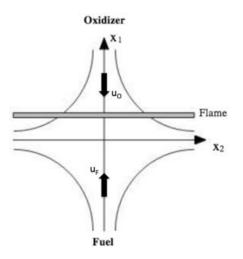
Figure 3.5: Canonical laminar stretched flame. Extracted from Poinsot & Veynante 197.
