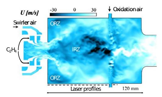
Fig. 3. ISF-3 Target Flame 1: Instantaneous axial velocity from LES in a mid-plane cut.
