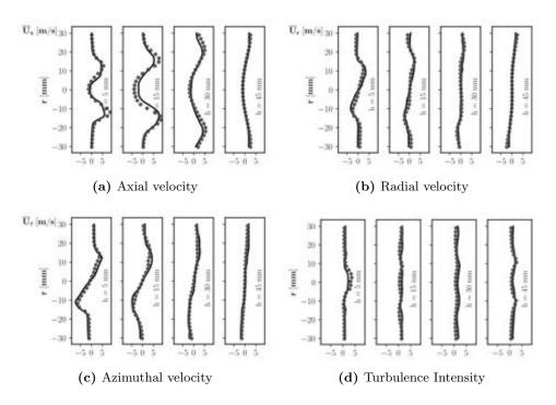
Figure 9.3: UTIAS configuration: Profiles of time-averaged velocity components and turbulent intensity at axial position 5mm, 15mm, 30mm and 45mm in non-reacting conditions. Symbols: experiment, black line: LES.
