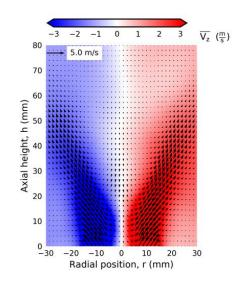
Figure 9.4: UTIAS configuration: Average axial velocity from LES in a mid-plane cut.
