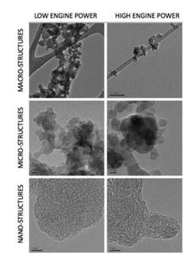
Figure 2.2: HRTEM images of derived soot macro - micro - and nano-structures; left column images are for low engine power level (4 - 7%) of the maximum thrust) and right column images are for high (maximum thrust)engine power. (Extracted from 46)
