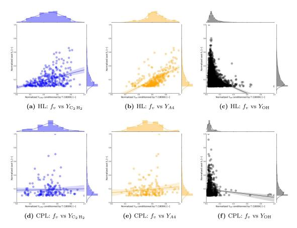
**Figure 8.36:** Scatterplots of soot volume fraction as a function of  $Y_{C_2H_2}$  (left),  $Y_{A4}$  (center) and  $Y_{OH}$  (right) conditioned on high temperature for RUN\_HL\_A4 (top) and RUN\_CPL\_A4 (bottom). Linear regressions highlight the dependencies.
