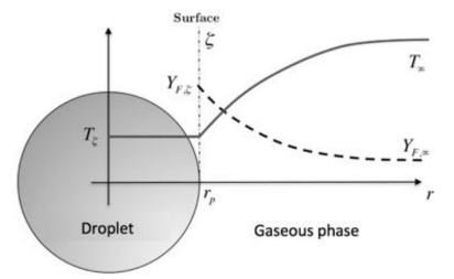
**Figure 3.8:** Radial profile of temperature T and fuel mass fraction  $Y_F$  around a droplet.
