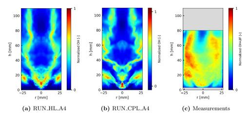
**Figure 8.12:** FIRST configuration: measured OH-LIF versus numerical normalized OH mass fraction field for cases RUN\_HL\_A4 (a) and RUN\_CPL\_A4 (b).
