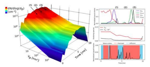
Figure 9.14: UTIAS configuration: a) PSDF evolution along the Lagrangian trajectory. b) Soot source terms (top), oxidizing species mass fractions (middle) and liquid volume fraction (bottom) along the particle trajectory.
