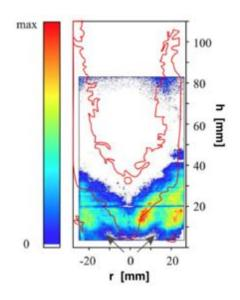
Figure 8.21: FIRST configuration: Average distribution of PAH measured by Laser Induced Fluorescence (LIF) and overlaid by red distribution isocontour ( $f_v > 0.1 \text{ } ppb$ , red line), extracted from [377].
