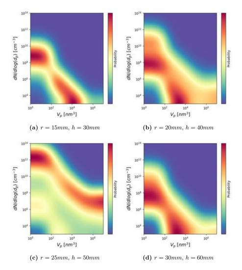
Figure 9.15: UTIAS configuration: Statistical PSDF at four locations.
