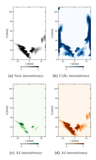
Figure 8.31: FIRST configuration: Soot and PAH intermittency over 20 ms for the case RUN\_HL\_A4 .
