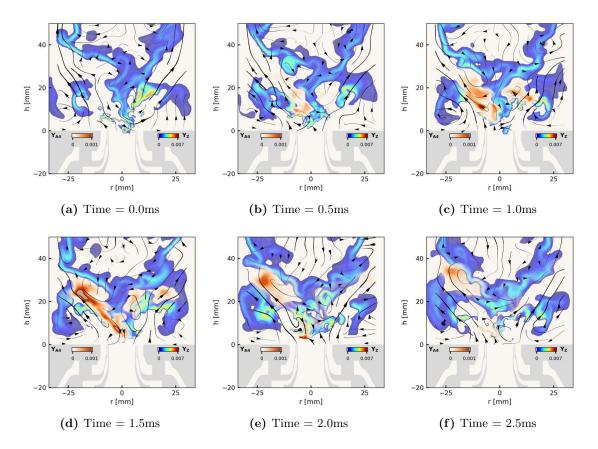
**Figure 8.28:** FIRST configuration: Sequence of OH mass fraction with overlaid orange A4 mass fraction, flow field velocity is represented by arrowed streamlines with a width proportional to the local velocity intensity for the case RUN\_HL\_A4.
