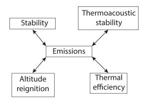
Figure 1.9: Design constraints applying to aeronautical burners.
