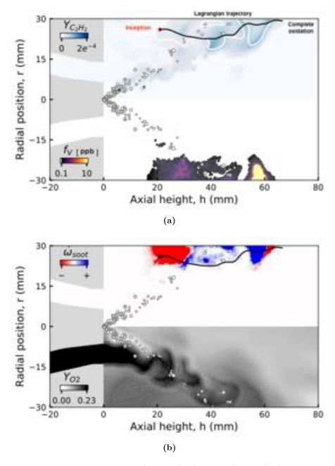
Figure 9.13: UTIAS configuration: a)  $C_2H_2$  (top) and  $f_v$  (bottom), b) soot source term (top) and  $O_2$  (bottom). In both images, the spray is represented by circles and one example of soot trajectory is shown.
