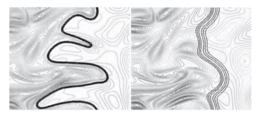
Figure 7.4: Flame-turbulence interaction for a thin and artificially thickened flame, studied by DNS [342].
