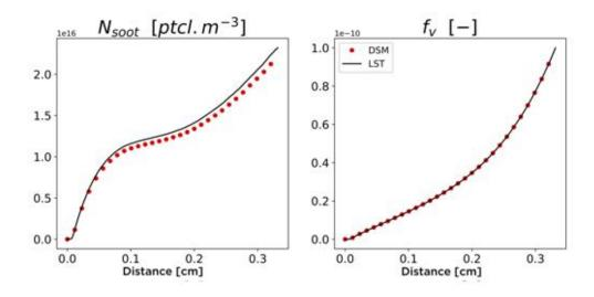
**Figure 6.3:** Comparison of soot number density and soot volume fraction between Lagrangian Soot Tracking (LST) and Discrete Sectional Method (DSM) on a freely propagating premixed flame considering only nucleation and coagulation .
