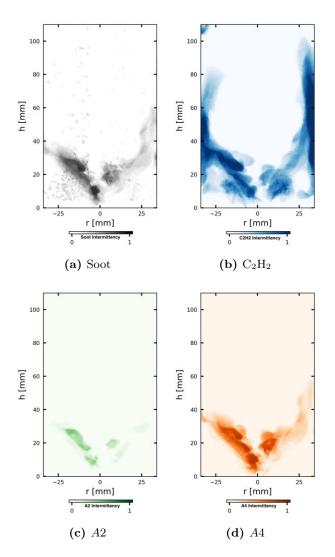
Figure 8.30: FIRST configuration: Soot and PAH intermittency over 20 ms for the case RUN\_HL\_A4 .
