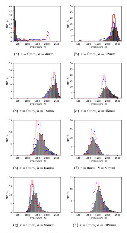
**Figure 8.8:** FIRST configuration: Probability Density Functions of temperature at various locations along the z-axis. Comparison between simulation with (red lines) and without (blue lines) thermal radiation, and CARS measurements (grey).
