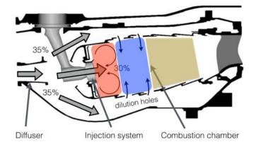
Figure 1.8: Sketch of a conventional RQL combustion chamber (Extracted from 20)
