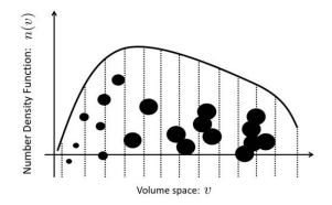
Figure 2.10: Soot number density function (NDF) over the volume described by soot particles.
