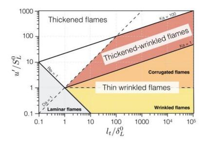
Figure 7.2: Combustion diagram for premixed turbulent combustion 334.
