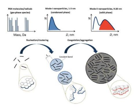
Figure 2.3: Schematic crystallite structure in soot nucleation and growth. (Extracted from 47)
