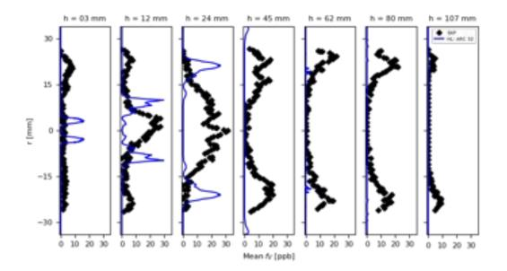
**Figure 8.24:** FIRST configuration: Radial mean  $f_v$  (blue line) compared with measurements (symbols) for the case RUN\_HL\_A4 : radial profiles at various heights.
