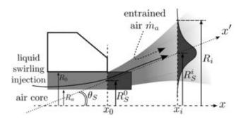
Figure 3.10: Scheme of the FIM-UR injection.
