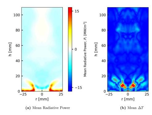
Figure 8.10: FIRST configuration: Mean Radiative Power (a) and and  $\Delta T$  (b) between cases with and without radiation (b).
