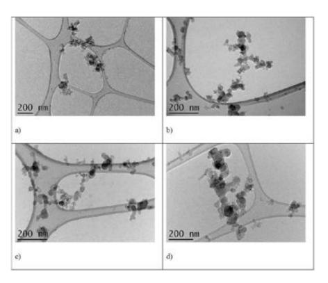
**Figure 2.1:** TEM images of soot aggregates emitted from a SaM146 engine at different thrust levels. a) 30% of the maximal thrust b) 70% of the maximal thrust c) 85% of the maximal thrust d) 100% of the maximal thrust. (Extracted from 18)
