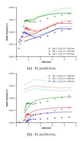
Figure 6.12: PAH predictions including soot consumption (dark) or not (light) in nucleation flames. Comparison between A2 and A4 measurements [285] and numerical approaches considering respectively C2H4\_A2\_28\_205\_14\_LG (lines) and C2H4\_A4\_32\_233\_13\_LG (dashed lines) chemical schemes.
