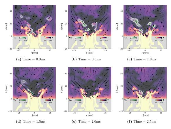
**Figure 8.27:** Case RUN\_HL\_A4 : Sequence of Temperature with overlaid green A2 mass fraction, flow field velocity is represented by arrowed streamlines with a width proportional to the local velocity intensity for the case RUN\_HL\_A4 .
