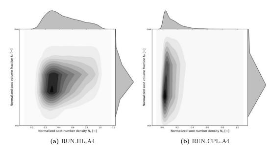
**Figure 8.37:** Joint PDF of soot volume fraction  $f_v$  as a function of soot number density  $N_s$  for the cases RUN\_HL\_A4 (a) and RUN\_CPL\_A4 (b).
