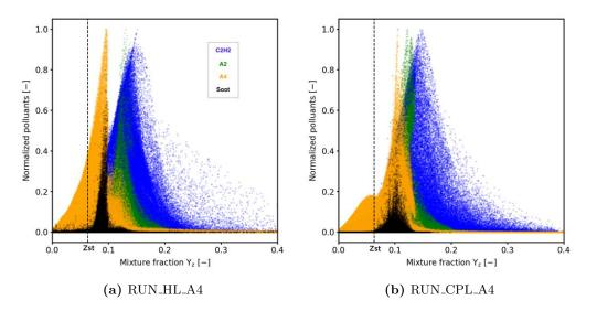
Figure 8.32: Scatterplots of soot volume fraction and precursors species as function of mixture fraction. Dashed line corresponds to the stoichiometric mixture fraction for the cases RUN\_HL\_A4 (a) and RUN\_CPL\_A4 (b).
