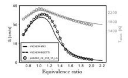
Figure 5.22: One-dimensional unstrained premixed laminar flames in the UTIAS Jet A-1 burner conditions [22]. Comparison of three chemical mechanisms in terms of laminar flame speed and adiabatic flame temperature.
