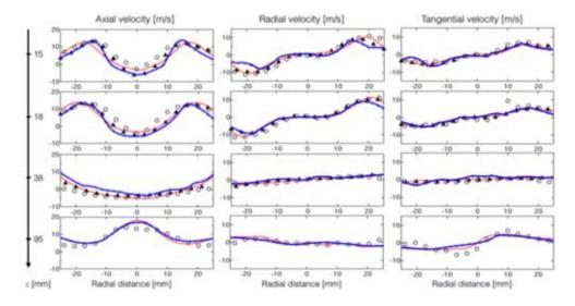
**Figure D.1:** FIRST configuration: Mean axial, radial and tangential velocity profiles for both chemical mechanisms extracted in mid-plane at z = 15, 18, 40 and 95 mm, RUN\_HL\_A4 (blue line), RUN\_CPL\_A4 (red line), experiment: FoV ( $\blacktriangle$ ) and SoC (o).
