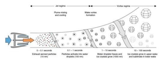
Figure 1.6: Processes influencing the contrail formation stage. (Extracted from 15)
