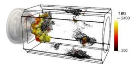
**Figure 8.23:** FIRST configuration: Instantaneous view of soot particles with an isovolume of heat release rate colored by the gaseous temperature for the case RUN\_HL\_A4 . Red circle highlights soot presence in the ORZ.
