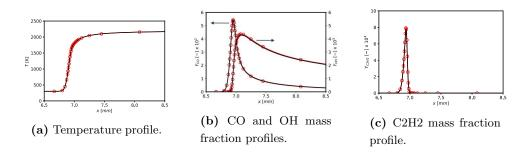
Figure 5.8: One-dimensional premixed unstrained ethylene-air laminar flame at P = 3 bars and equivalence ratio  $\phi = 0.8$ . Comparison between BISETTI (----), C2H4\_A2\_28\_205\_14\_LG (O). of T (a), CO and OH (b) and C\_2H\_2 (c).
