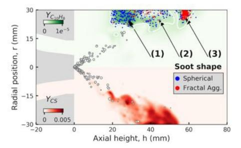
Figure 9.10: UTIAS configuration: Instantaneous field of naphthalene mass fraction (top) with overlaid iso-contours of soot nucleation and soot particles. Instantaneous  $Y_{CS}$  field (bottom) with some droplets represented by circles.
