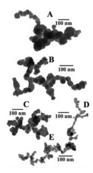
Figure 2.4: TEM images of soot aggregates at 2.3 atm (A), 4 atm (B), 5.4 atm (C), 7.1 atm (D), and 10 atm (E). (Extracted from 55)
