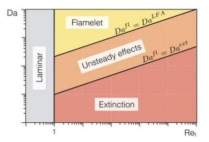
Figure 7.3: Combustion diagram for non-premixed turbulent combustion 336.
