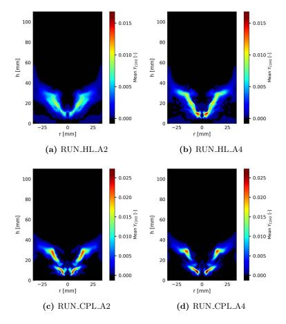
Figure 8.18: FIRST configuration: Numerically predicted  $C_2H_2$  mass fraction for the 4 simulations.
