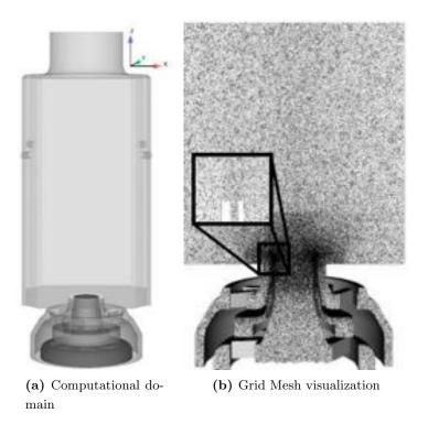
Figure 8.2: Computational domain and mesh of FIRST configuration.
