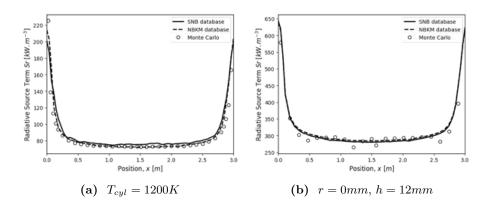
**Figure B.1:** RTC1: Comparison between SNB, new NBKM spectral database against the reference Monte-Carlo method using line-by-line model.
