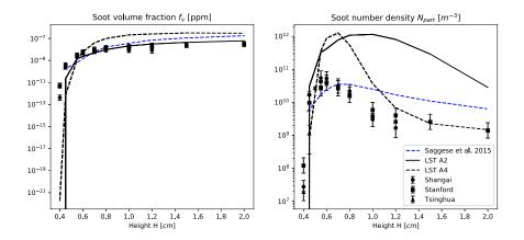
Figure 6.14: Soot prediction in ISF Premixed Flames 6. Comparison between experiments [331], numerical approaches from literature [108] and Lagrangian Soot Tracking with different soot precursors species.
