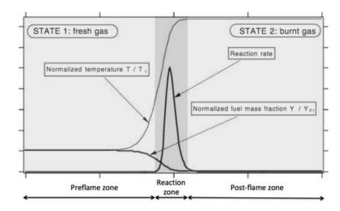
Figure 3.1: Laminar premixed flame structure. Extracted from Poinsot & Veynante 197.
