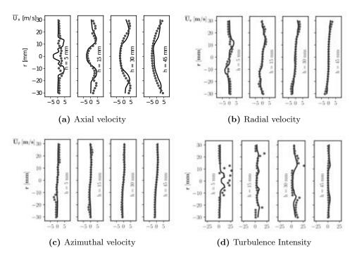
Figure 9.8: UTIAS configuration: Profiles of time-averaged mean velocity and turbulent intensity at axial position 5mm, 15mm, 30mm and 45mm in reacting conditions. Symbols: experiment, black line: LES.
