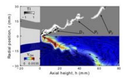
Figure 9.7: UTIAS configuration: Instantaneous Takeno Index conditionned by heat release rate (top) and OH mass fraction with superimposed streamlines (bottom).
