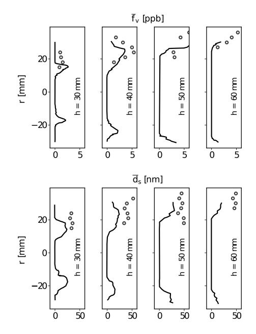
Figure 9.9: UTIAS configuration: Radial profiles of mean soot volume fraction (top) and mean soot primary diameter (bottom) at four axial positions: LES (line) vs LII measurements (symbols).
