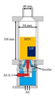
**Figure 9.1:** UTIAS configuration: Cross-sectional view of the burner assembly. Yellow box indicates the region mapped by the SPIV planar measurement, and dark blue box shows the region probed by the LII point measurement. (from [22]).
