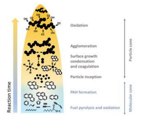
Figure 2.7: Schematic representation of soot evolution. (Adapted from 66)
