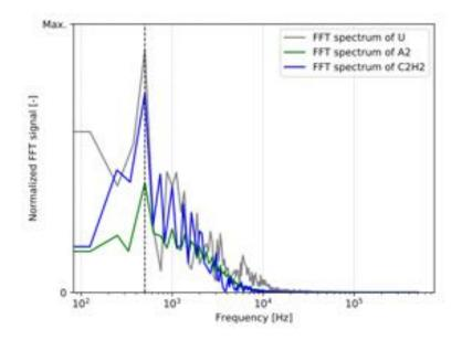
**Figure 8.26:** Case RUN\_HL\_A4 : Fast Fourier Transform at a probe location close to the injector (r = 4mm, h = 3mm).
