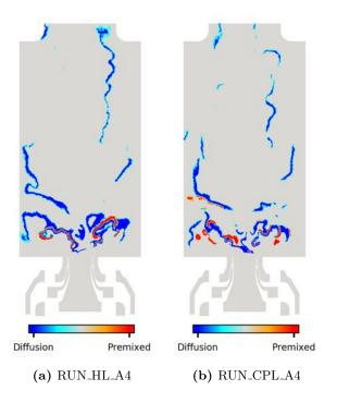
Figure 8.14: FIRST configuration: Takeno Index computed based on CO.
