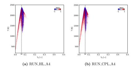
Figure 8.16: FIRST configuration: Scatterplots of temperature as a function of mixture fraction colored by the Takeno Index in the dilution zone for cases RUN\_HL\_A4 (a) and RUN\_CPL\_A4 (b).
