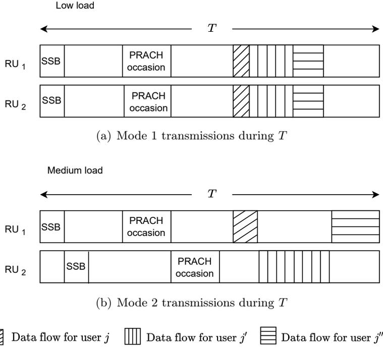
Figure 6.1: SSB, PRACH, and data transmissions/receptions over  $T$ .
