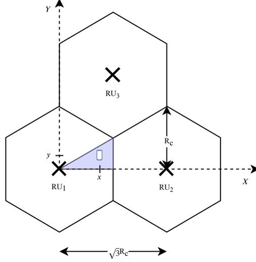
Figure 3.6: Zone of study in the hexagonal cell.
