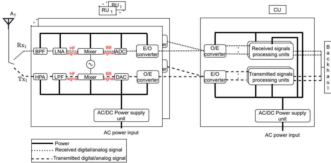
Figure 6.2: Power-consuming units in a C-RAN architecture.
