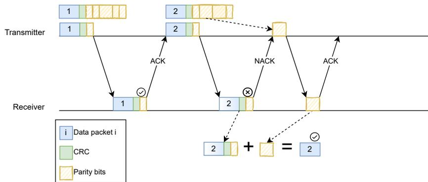
Figure 2.6: HARQ-IR diagram.
