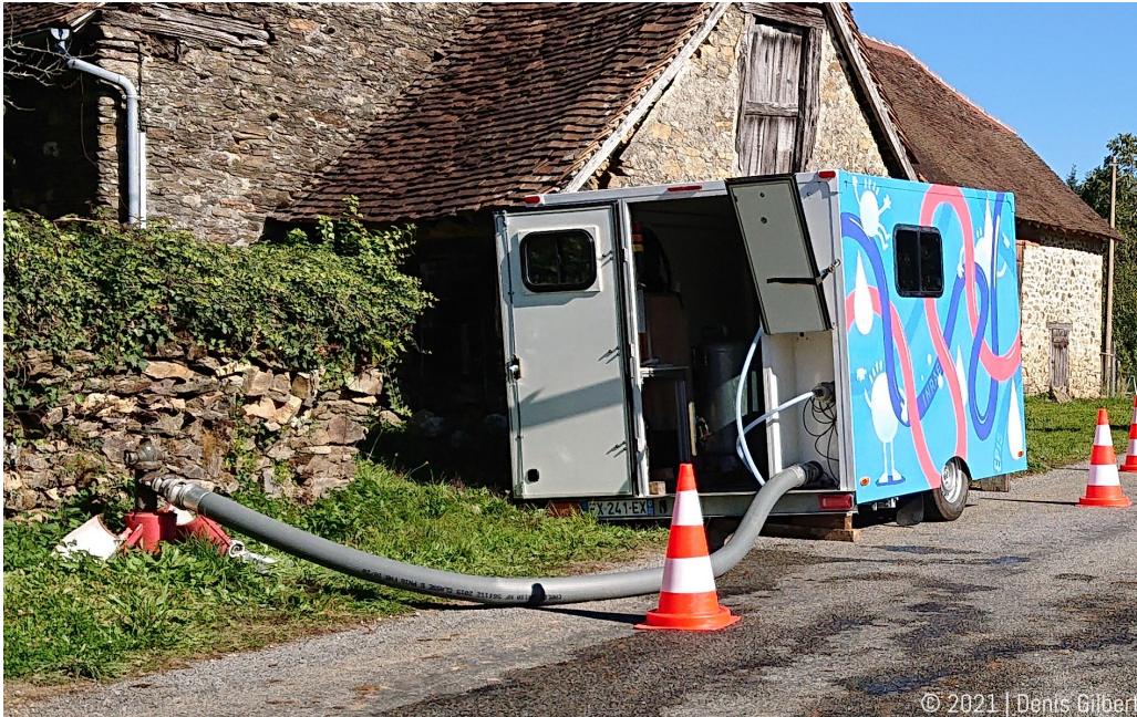
Figure 5.1: Mobile measuring device connected to a fire hydrant, designed by [52]; this device is called “the Trailer” in all current chapter.
