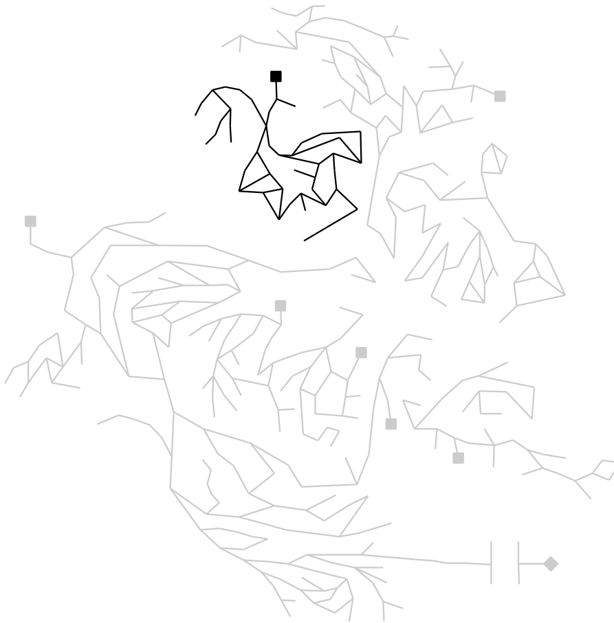
Figure 4.4: In black: district metered area (DMA) of the adapted network C-Town, used to simulate inertia phenomena. In gray: other DMAs (not used). The \blacksquare / \square represent the tanks. The \blacklozenge represents a reservoir.
