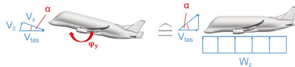
Figure 3.5: Heave, pitch and vertical gust modes at a frequency close to zero (source:[17])
