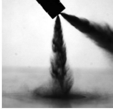
Figure 1. GDI spray impinging upon a smooth plate. Fuel pressure is 100bar.
