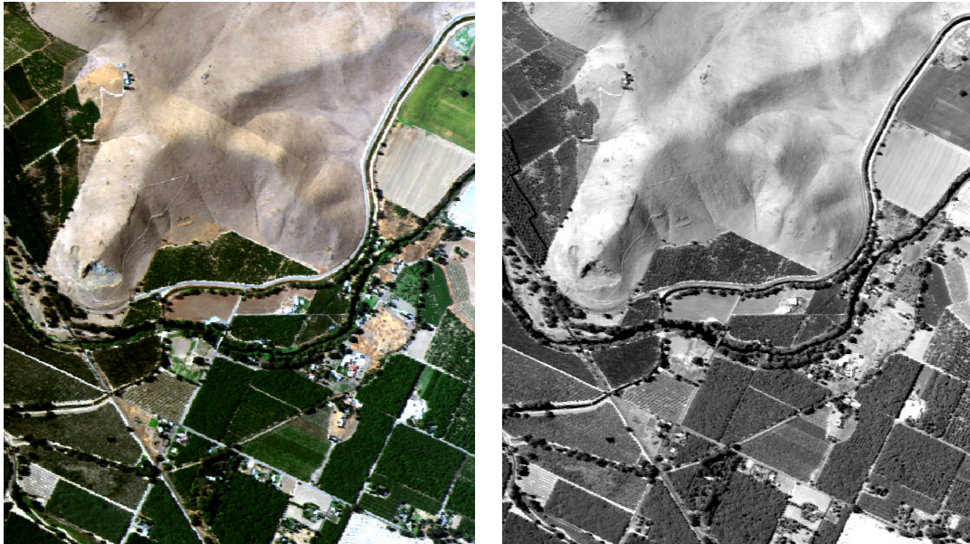
Figure 3.6.: AVIRIS image: color composition of hyperspectral image (left) and corresponding panchromatic image (right).
