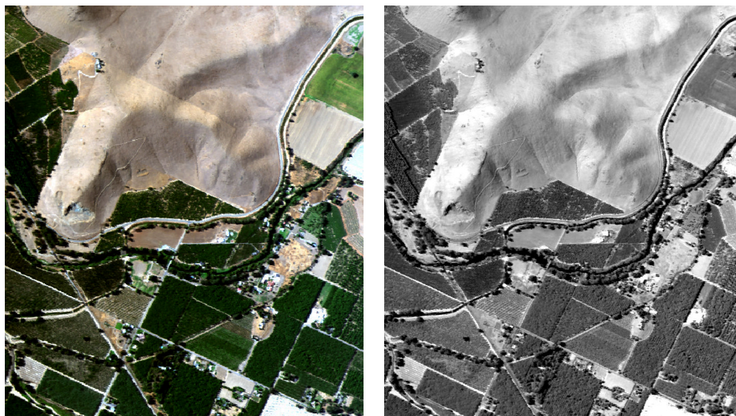
Figure 3.6.: AVIRIS image: color composition of hyperspectral image (left) and corresponding panchromatic image (right).
