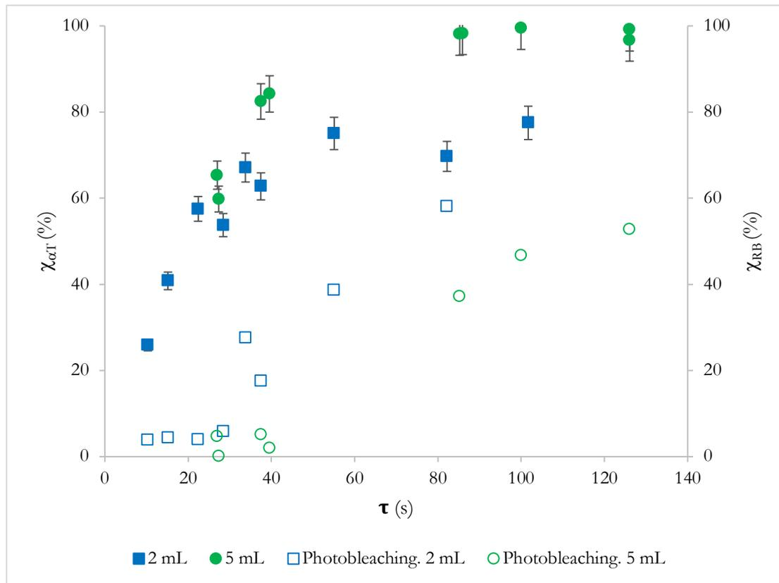
**Figure 4.4.** Photoreactor *Vapourtec*. Variation of the conversion in  $\alpha T$  (%) and of the photobleaching rate  $\chi_{RB}$  (%) with the residence time  $\tau$  (s) for two different reactor volumes ( $V_{Ph_1} = 5$  mL and  $V_{Ph_2} = 2$  mL) and for fixed  $q \approx 5$  and  $f \approx 1.5$ .  $C_{\alpha T,0} = 0.037$  mol.L<sup>-1</sup> and  $C_{RB,0} = 4.0 \times 10^{-5}$  mol.L<sup>-1</sup>.
