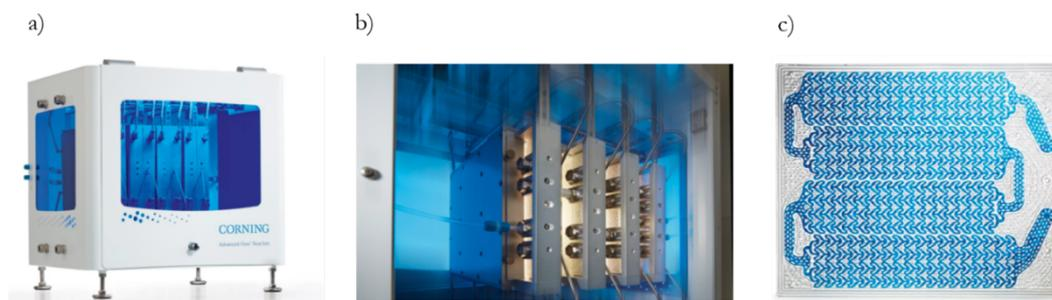
**Figure 2.17.** Photography of the G3 Photo Reactor a), b) (from [www.corning.com](http://www.corning.com)) and of a fluidic module of the G3 Photo Reactor c) (from [www.corning.com](http://www.corning.com)).
