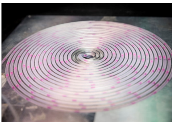
Figure 2.6. Images of the spiral-shaped reactor [Jean-Claude Moschetti, LGC, CNRS Photothèque].
