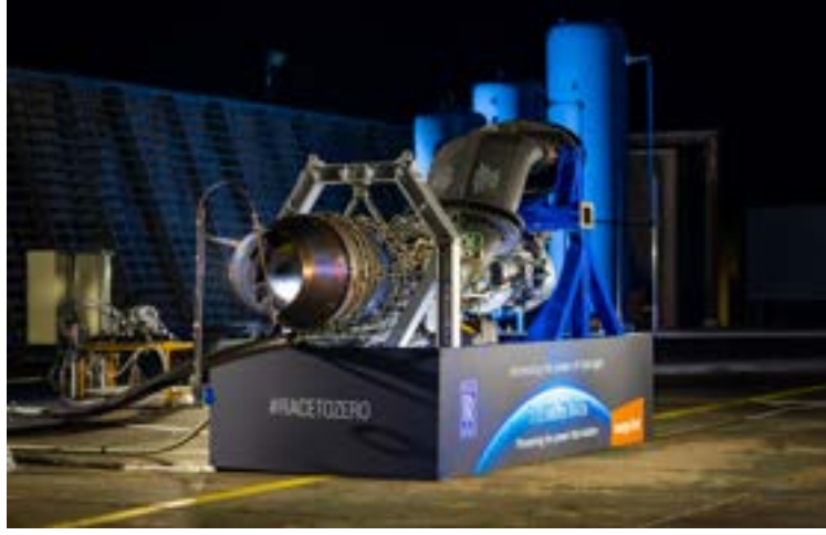
Figure 1.8 – Adapted Rolls-Royce AE 2100-A regional aircraft engine for hydrogen combustion recently tested by Rolls Royce in collaboration with EasyJet [13].
