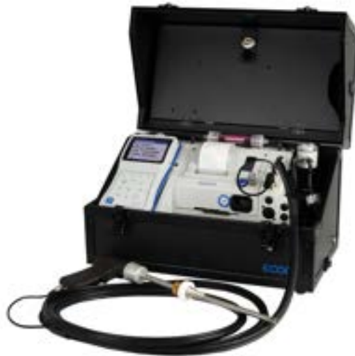
Figure 2.30 – ECOM J2KN flue gas analyzer.
