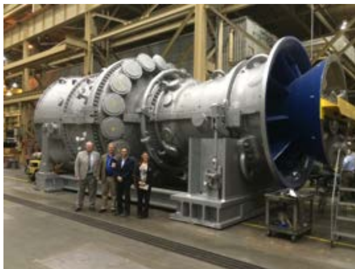
Figure 1.5 – Illustration of the CAN-annular General Electric 9F.03 gas turbine producing 265 MW electrical power.
