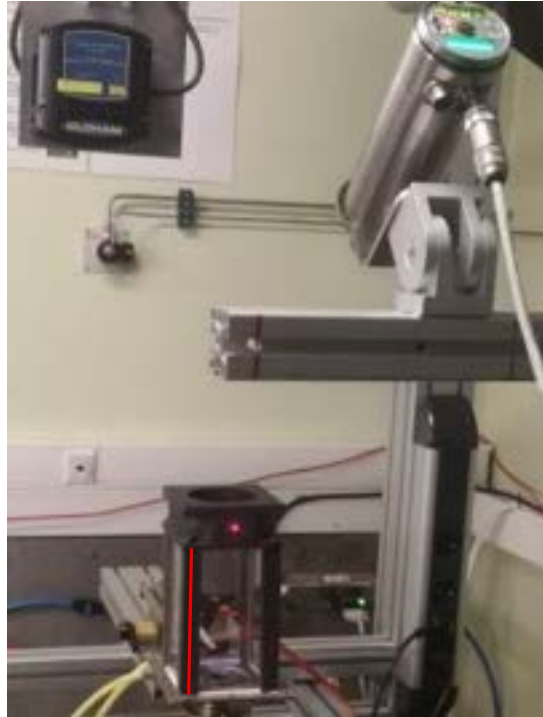
Figure 2.22 – Double wavelength pyrometer installed for the measurement of the surface temperature of the convergent section at the top of the combustion chamber during operation with a hydrogen/air flame.
