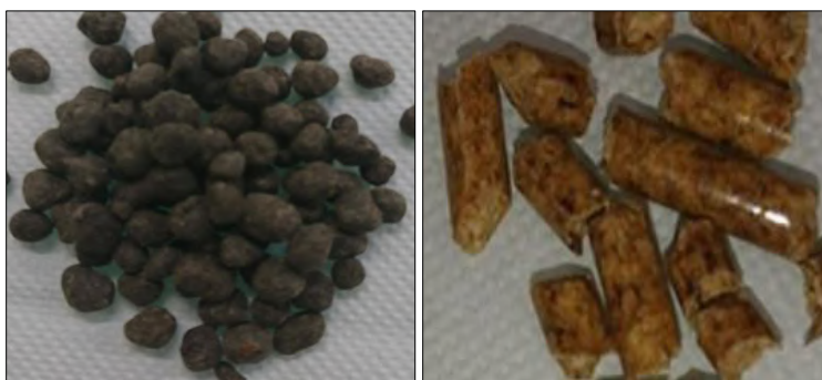
Figure 3.2 : Picture of original fuel, (left) Aerobic sewage sludge, (Right) pine softwood pellet.
