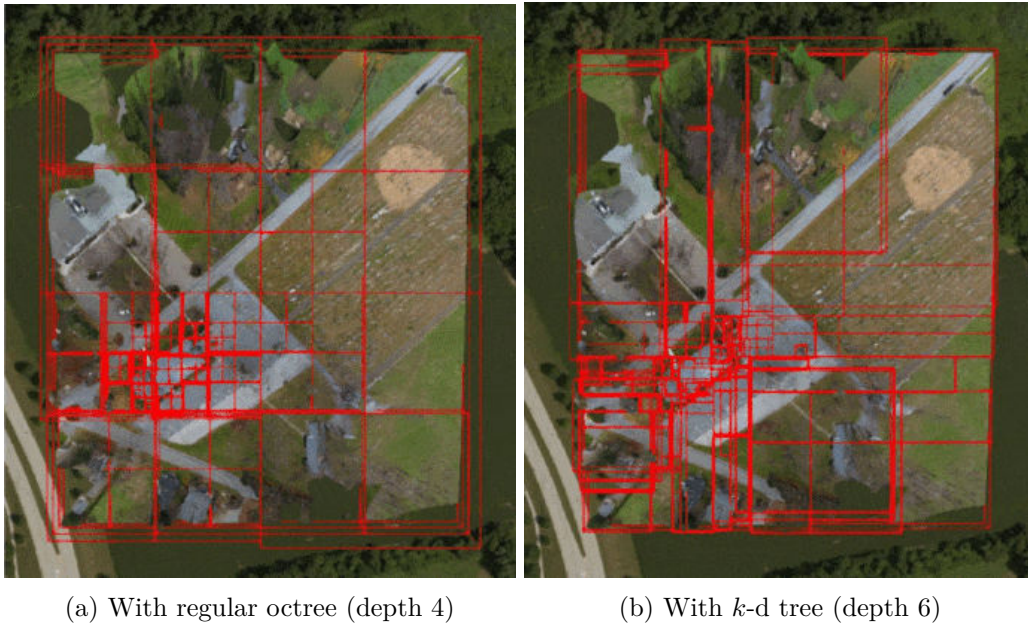
Figure 2.6: Spatial partitioning used in 3D Tiles
