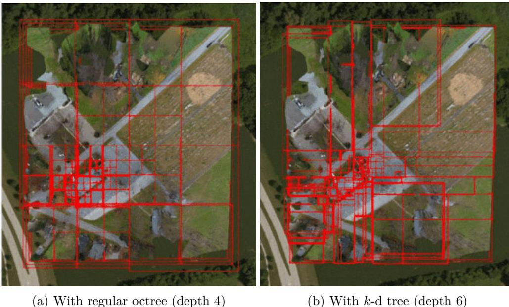
Figure 2.6: Spatial partitioning used in 3D Tiles
