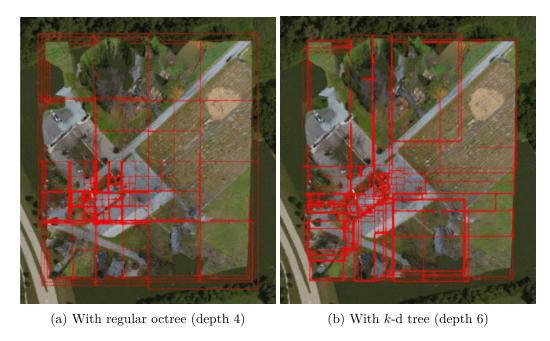
Figure 2.6: Spatial partitionning used in 3D Tiles
