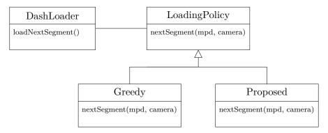
Figure 4.5: Class diagram of our DASH client
