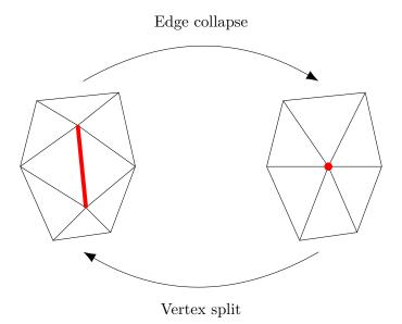
Figure 2.2: Vertex split and edge collapse
