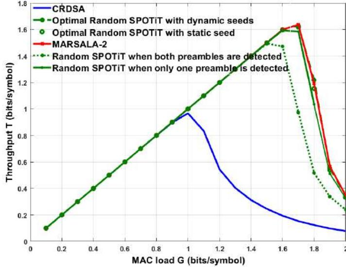
Figure 3.5: Throughput comparison between R-SPOTiT, MARSALA-2 and CRDSA,  $E_S/N_0 = 10$  dB, 100 slots per frame, QPSK modulation, Turbo coding of rate 1/3 and equipowered packets of 100 bits and  $N_R = 2$  replicas per packet.
