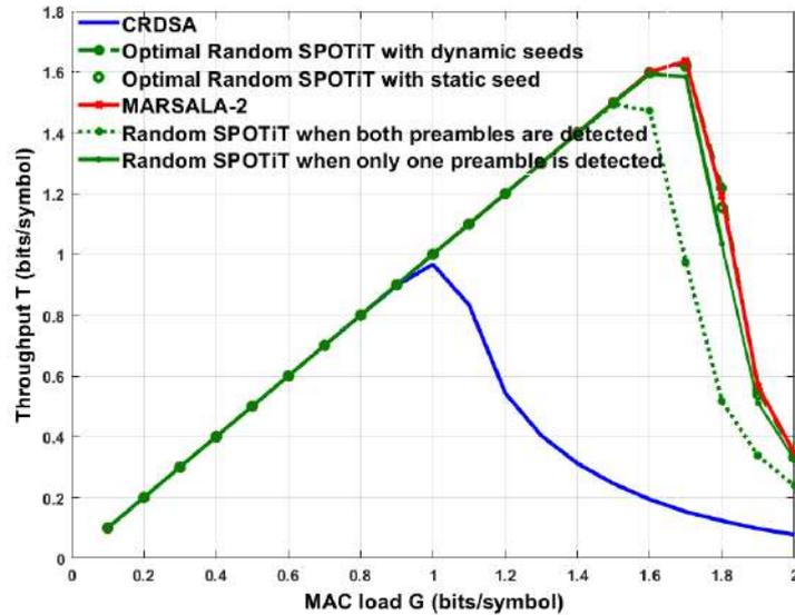
Figure 9.3: Throughput comparison between R-SPOTiT, MARSALA-2 and CRDSA,  $E_S/N_0 = 10$  dB, 100 slots per frame, QPSK modulation, Turbo coding of rate 1/3 and equipowered packets of 100 bits and  $N_R = 2$  replicas per packet.
