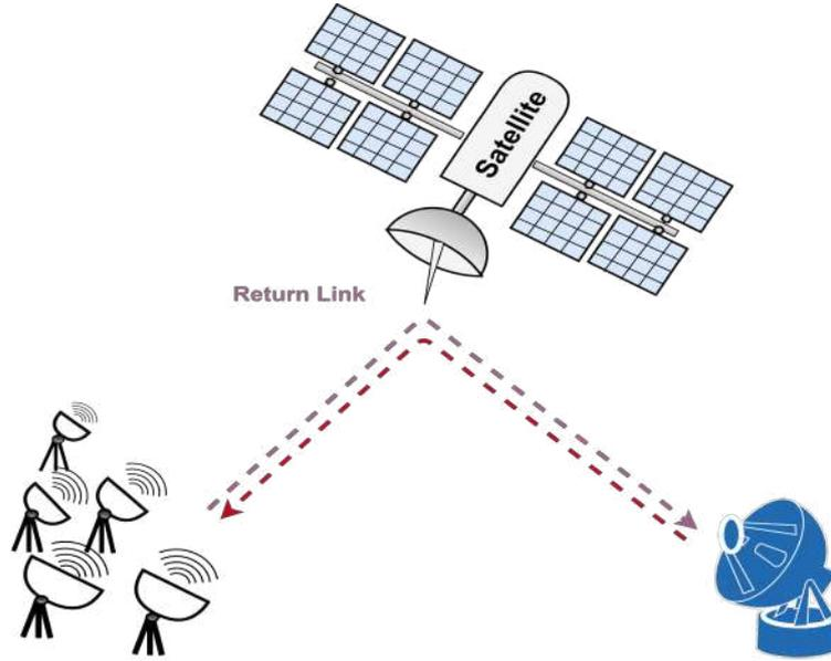
Figure 3.1: Satellite communication system example with a bent pipe satellite.
