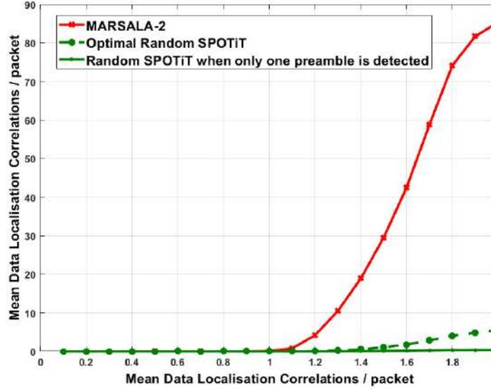
Figure 3.7: Complexity of MARSALA-2 vs R-SPOTiT in terms of localization correlations,  $E_S/N_0 = 10$  dB, 100 slots per frame, QPSK modulation, Turbo coding of rate 1/3 and equipowered packets of 100 bits.
