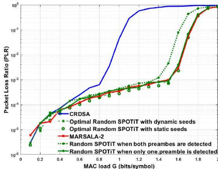
Figure 9.4: Packet Loss Ratio comparison between R-SPOTiT, MARSALA-2 and CRDSA,  $E_S/N_0 = 10$  dB, 100 slots per frame, QPSK modulation, Turbo coding of rate 1/3 and equipowered packets of 100 bits and  $N_R = 2$  replicas per packet.
