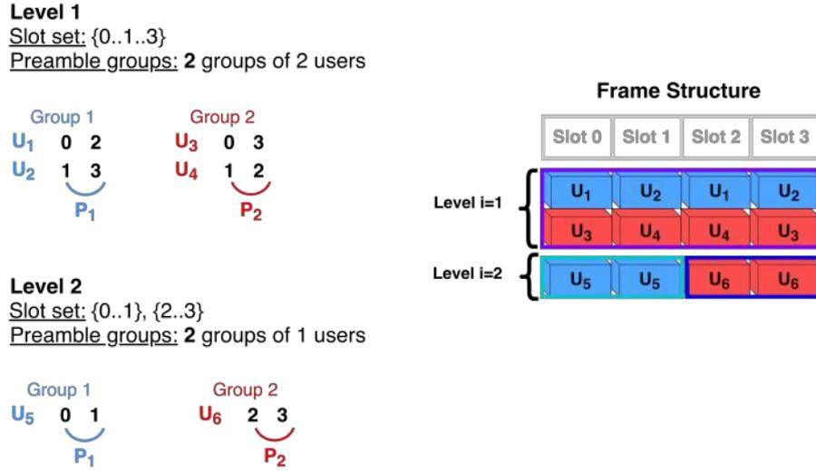
Figure 5.1: Optimal frame structure,  $N_S = 4$ ,  $N_R = 2$ ,  $N_P = 2$ .
