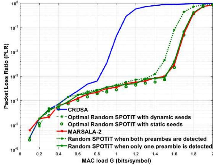
Figure 3.6: Packet Loss Ratio comparison between R-SPOTiT, MARSALA-2 and CRDSA,  $E_S/N_0 = 10$  dB, 100 slots per frame, QPSK modulation, Turbo coding of rate 1/3 and equipowered packets of 100 bits and  $N_R = 2$  replicas per packet.
