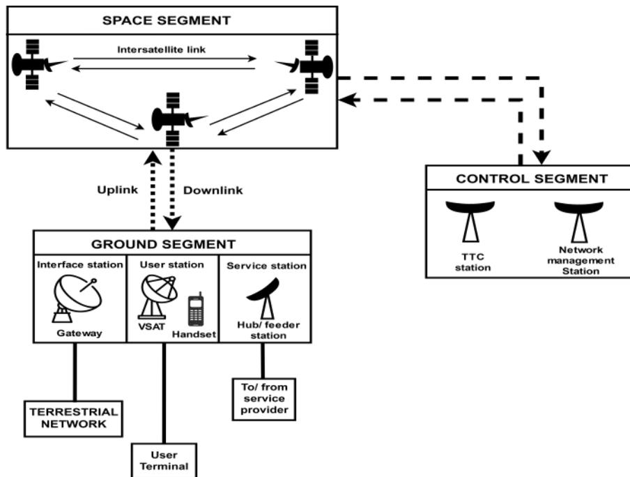
Figure 2.1: Overview of a satellite communication system interfacing with terrestrial entities.
