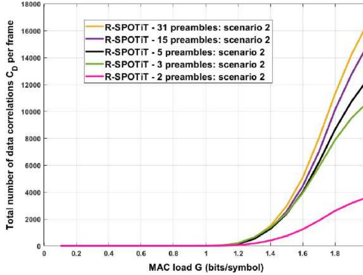
Figure 4.12: Data detection complexity in case of multi-preamble R-SPOTiT
