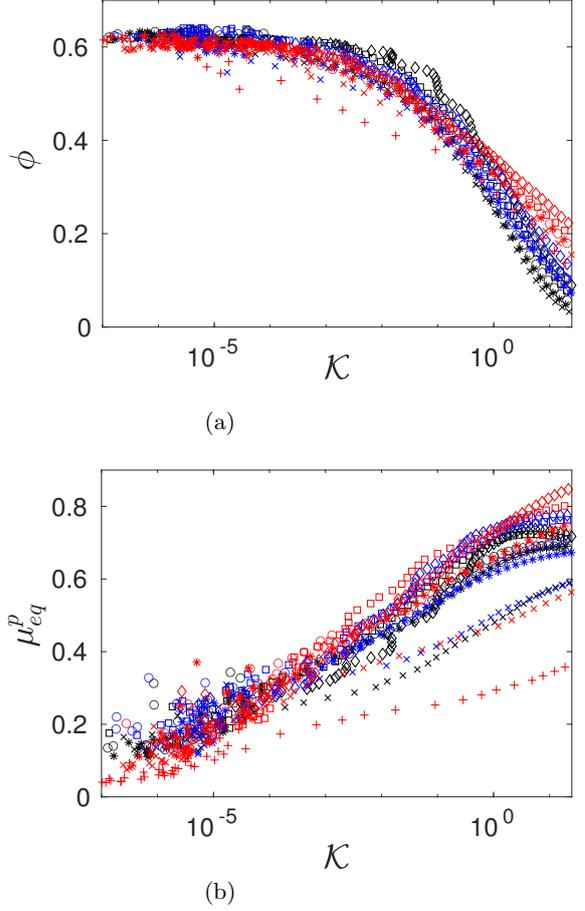
FIG. 11. Constitutive laws  $\phi(\mathcal{K})$  and  $\mu_{eq}^p(\mathcal{K})$  of the equivalent granular phase for all the cases considered in the present work: (black)  $Re_p = 0.1$ ; (blue),  $Re_p = 1$ ; (red),  $Re_p = 10$ . The various symbols indicate various  $\theta$  as in figure 8(a).
