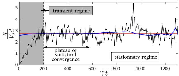
FIG. 2. (Colour online) Time evolution of the instantaneous granular flow rate per unit depth scaled by  $V_s$  with  $V_s = (\rho_p - \rho_f)gd^2/(18\eta_f)$  the Stokes velocity ( $Re_p = 1$ ,  $\theta = 0.67$ ). Black line: IBM-DEM results. Red line: mean value at steady state. Blue line:  $f_{conv}$  defined in (8) used to check time convergence (here,  $t_{max} = 1300\dot{\gamma}^{-1}$ ).
