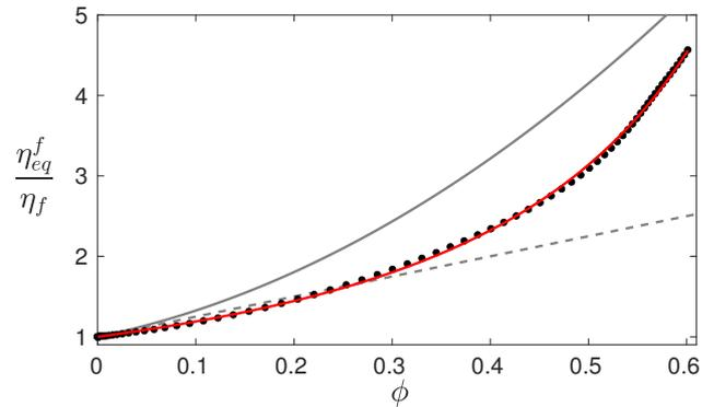
FIG. 7. Apparent viscosity  $\eta_{eq}^f / \eta_f$  of the fluid phase vs. solid volume fraction  $\phi$ : (•), present IBM-DEM simulation for  $Re_p = 1$ ,  $\theta = 0.67$  (eq. (44)); (dashed black), Einstein's model [8, 9]  $\eta_{eq}^f / \eta_f = 1 + \frac{5}{2}\phi$ ; (solid black), Gibilaro et al. (2007)'s correlation [11]  $\eta_{eq}^f / \eta_f = (1 - \phi)^{-\beta}$  with  $\beta = 2.8$ ; (red), adjustment with  $\eta_{eq}^f / \eta_f = (1 - \phi)^{-1.65}$ .
