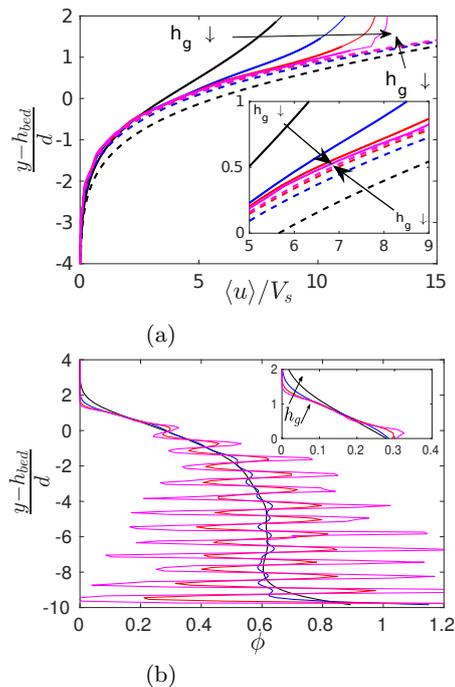
FIG. 18. (a) Velocity profile of the fluid phase (dashed) and the granular phase (solid) for various of  $h_g = \{d/10, d/4, d/2, 1\}$ . Velocity is scaled by  $V_s$  with  $V_s = (\rho_p - \rho_f)gd^2/(18\eta_f)$  the Stokes velocity. (b) Solid volume fraction  $\phi$  for the same values of  $h_g$ .
