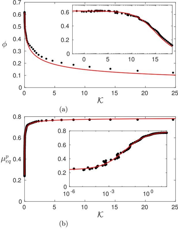
FIG. 10. Constitutive law of the equivalent granular phase ( $Re_p = 1$ ,  $\theta = 0.67$ ). (a) Solid volume fraction  $\phi$  versus  $\mathcal{K}$ , (b) Apparent friction coefficient  $\mu_{eq}^p$  versus  $\mathcal{K}$ : ( $\bullet$ ), present IBM-DEM simulation; (red),  $\phi(\mathcal{K})$  and  $\mu_{eq}^p(\mathcal{K})$  given by (33) and (35), respectively, with  $\phi_c = 0.615$ ,  $\mu_1 = 0.243$ ,  $\mu_2 = 0.794$  and  $\sqrt{K_0} = 0.125$ . Insets: semi-log representation.
