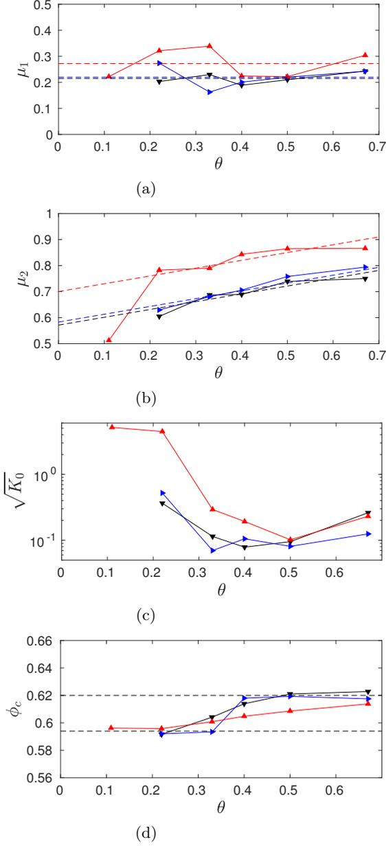
FIG. 12. Evolution of the parameters used in the model (33)-(35) of [13] as a function of  $\theta$  and  $Re_p$ : ( $\blacktriangledown$ ),  $Re_p = 0.1$ ; ( $\blacktriangleright$ ),  $Re_p = 1$ ; ( $\blacktriangle$ ),  $Re_p = 10$ . The dashed lines represent (a)  $\mu_1 \simeq 0.214 + 5.78 \times 10^{-2} Re_p$ ; (b)  $\mu_2 \simeq 0.57 + 0.30 \theta + 1.3 \times 10^{-2} Re_p$ ; (d),  $0.59 \leq \phi_c \leq 0.62$ .
