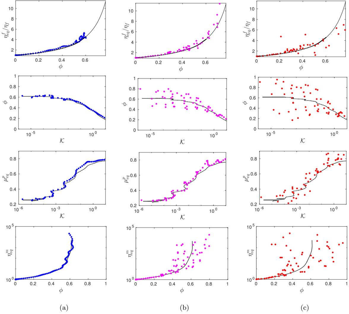
FIG. 19. Apparent rheology of the mesoscopic fluid phase (top row), granular phase (second and third rows) and mixture phase (bottom row): (a, blue),  $h_g = d/2$ , (b, magenta),  $h_g = d/4$ ; (c, red),  $h_g = d/10$ . Results for  $h_g = d$  are also plotted as reference (black). For the apparent viscosity of the fluid phase, the model  $\eta_{eq}^f/\eta_f = (1 - \phi)^{-1.65}$  is also plotted (solid black line).
