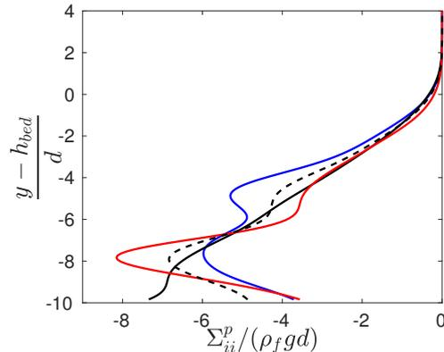
FIG. 9. Vertical distribution of the normal components of the equivalent granular phase ( $Re_p = 1$ ,  $\theta = 0.67$ ): (solid black),  $\Sigma_{yy}^p$ ; (blue),  $\Sigma_{xx}^p$ ; (red),  $\Sigma_{zz}^p$ ; (dashed black),  $P^p = (\Sigma_{xx}^p + \Sigma_{yy}^p + \Sigma_{zz}^p)/3$ .
