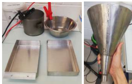
Figure 2.14: Metal cups and funnel used to reduce electrostatic charges
