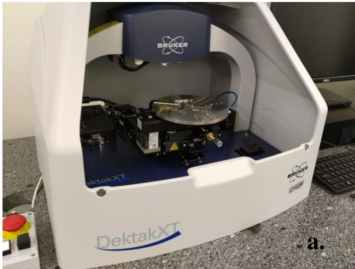
Fig 2.17: Mechanical profilometer (Dektak XT, Bruker) in ESIEE Paris' cleanroom. Picture a shows the whole equipment; b is a zoom on the stylus.
