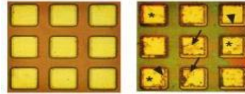
Fig 1.21: Example of a material failure. Degraded gold electrodes after eight months implanted in rat eye (Chow et al., 2001).
