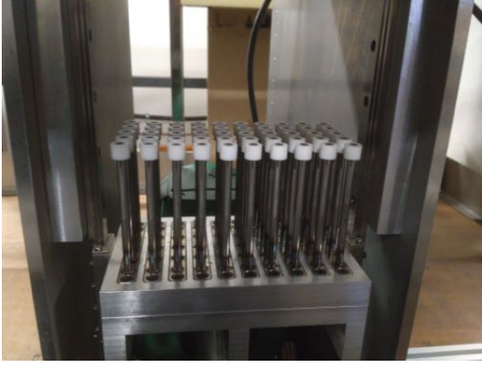
(a) Overview of the 50 pipes used as cavities to extend the plate perforations, with pistons underneath.
