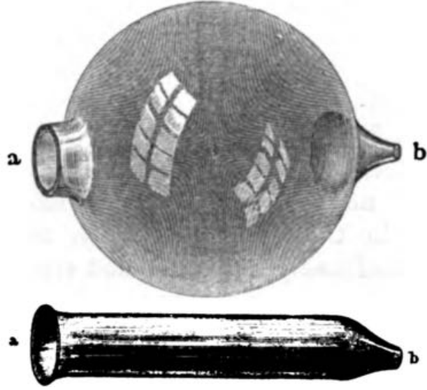
Figure 1.2: Scheme of resonators designed by Helmholtz [17]; (a): funnel shaped opening, for insertion into the ear; (b): sharp edges opening, neck
