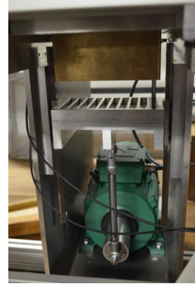
(b) Overview of the engine used to move the pistons.
