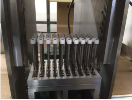
(a) Overview of the 50 pipes used as cavities to extend the plate perforations, with pistons underneath.
