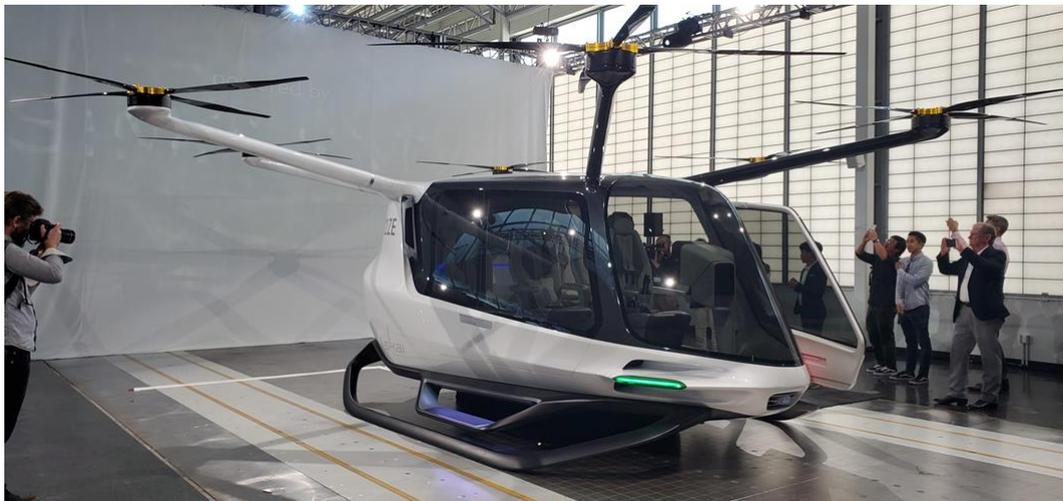
Fig. I-46: Alaka'i Skai Hydrogen powered VTOL air taxi[61].
