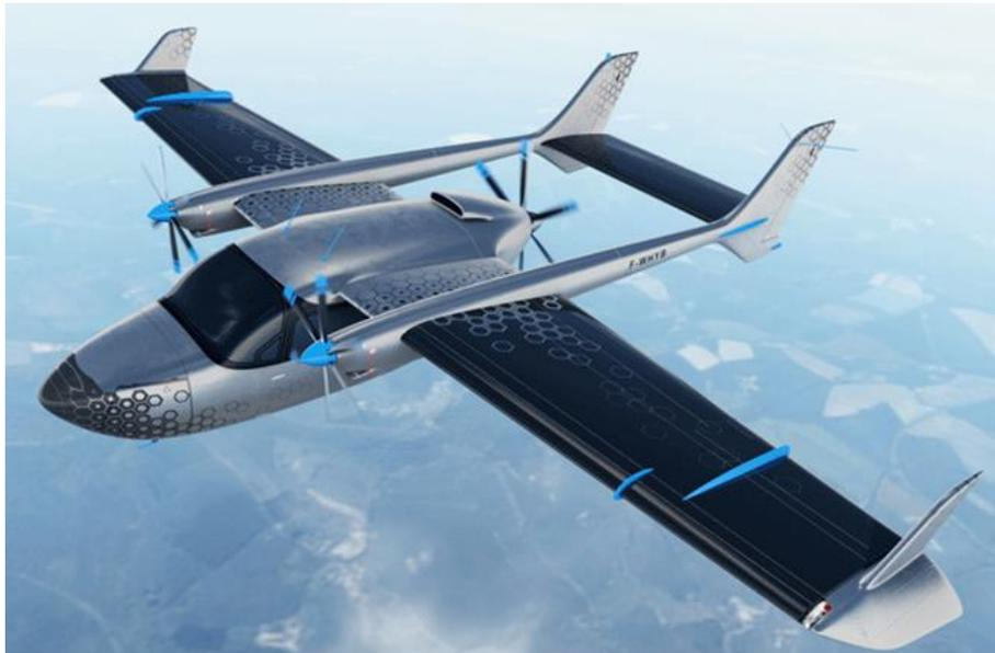
Fig. I-27: VOLTAERO Cassio hybrid-electric aircraft.
