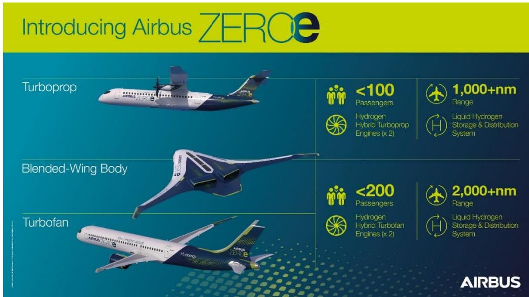
Fig. I-45: Airbus ZEROe aircraft concepts[60].
