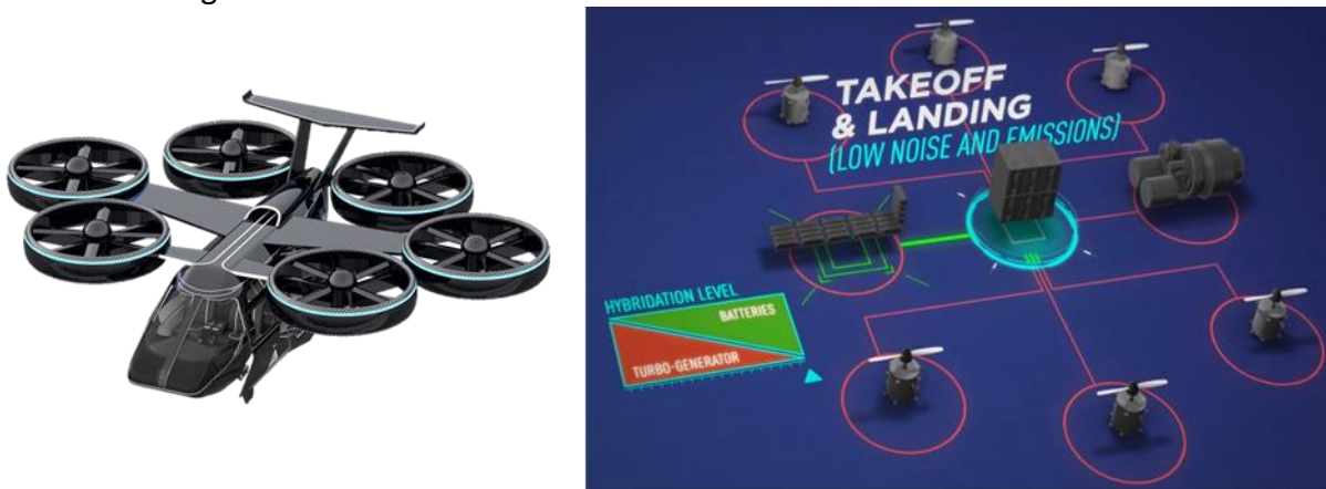
Fig. I-32: VTOL Bell NEXUS propulsive system description from SAFRAN [45].
