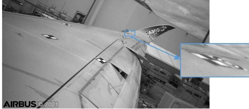
Figure 2.15: Example of view on an A350 wing using a 4K camera, with concentric circular and cross targets installed.
