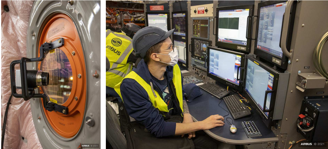
Figure 4.1: Cabin installation of the cameras. (a) - Camera mounted on a fake window, (b) - Station of the flight test engineers, used to control the recordings.
