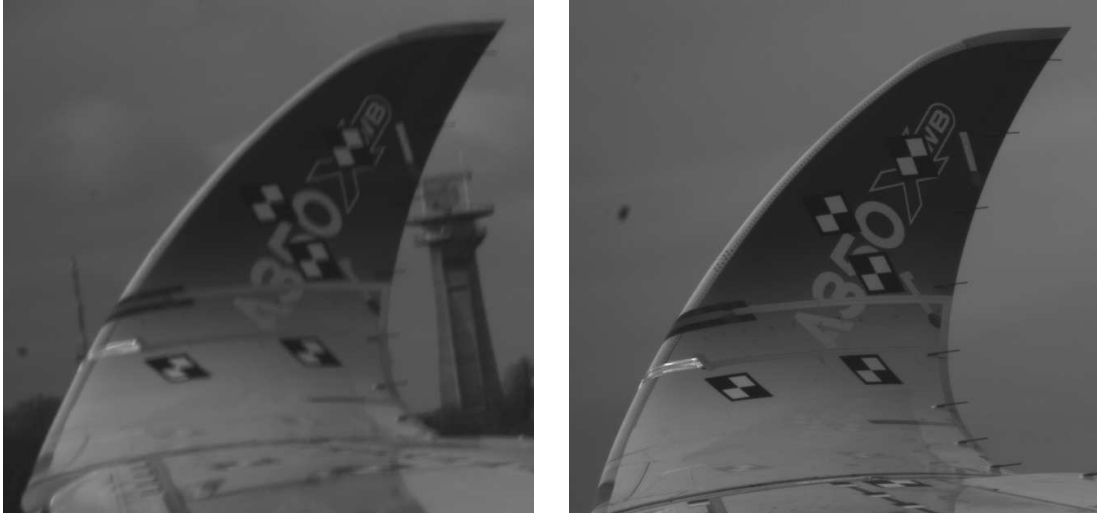
Figure 4.5: Examples of blur occurring on ground displacements. (a) - Image of the wing tip during landing, (b) - same view during flight.
