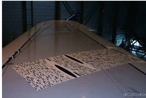
Figure 1.14: Example of pattern stripe installed for IPCT tests for an A380 in 2009.
