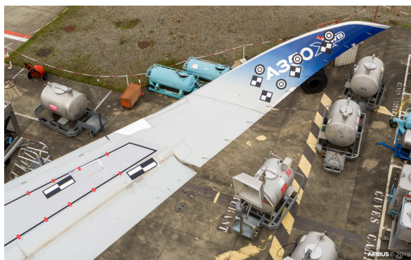
Figure 2.16: Selected targets installed on an A350 wing, with red graduations stuck on the black lanes.
