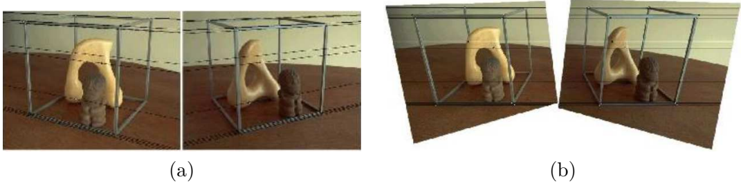
Figure 2.11: Example of stereo image rectification (from [LZ99]). (a) - Pair of initial images, (b) - Rectified images.
