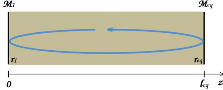
Figure 1.16: Schema of Fabry-Perot Laser Cavity, Equivalent Mirror Model
