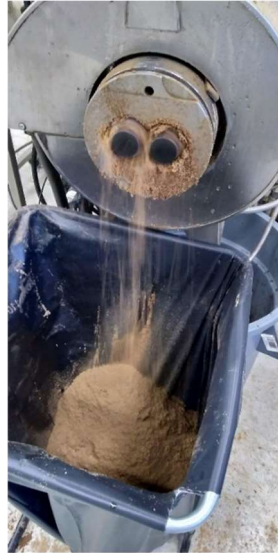
Figure 40. Extrudate obtained by twin-screw extrusion of teak sawdust using an extruder BC45 (Clextal, France)
