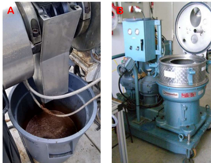
Figure 39. A: filtrate obtained by twin-screw extrusion of teak sawdust using an extruder BC45 (Clextral, France). B: centrifuge (Rousselet)
