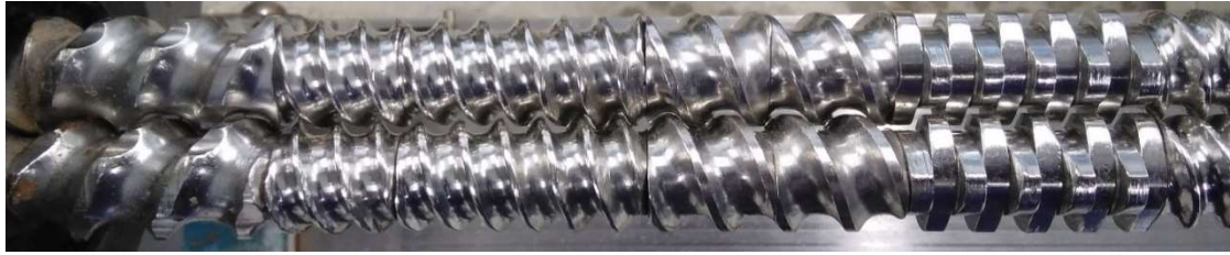
Figure 8. Twin-screw profile, from left to right reverse, conveying and kneading elements
