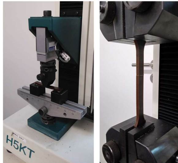
Figure 72. Flexural test (left) and tensile test (right) with a universal testing machine (Tinius Olsen H5KT)
