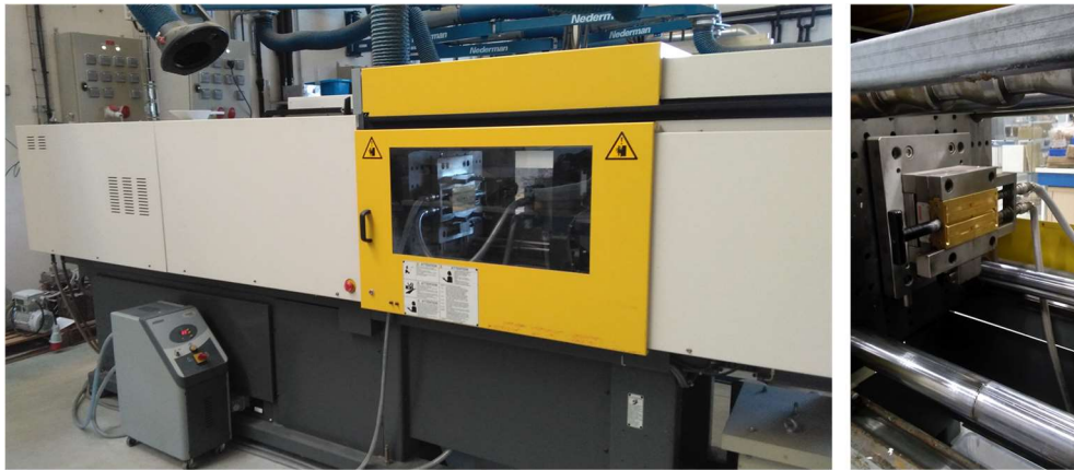
Figure 69. Injection-molding machine (FANUC Series 180is-IB) (left) and clamping unit with mold for flexural test specimens (right)
