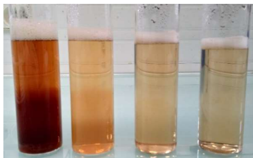
Figure 17. Aqueous extraction of teak sawdust using an ASE system, from left to right at 30 min, 60 min, 90 min, and 120 min
