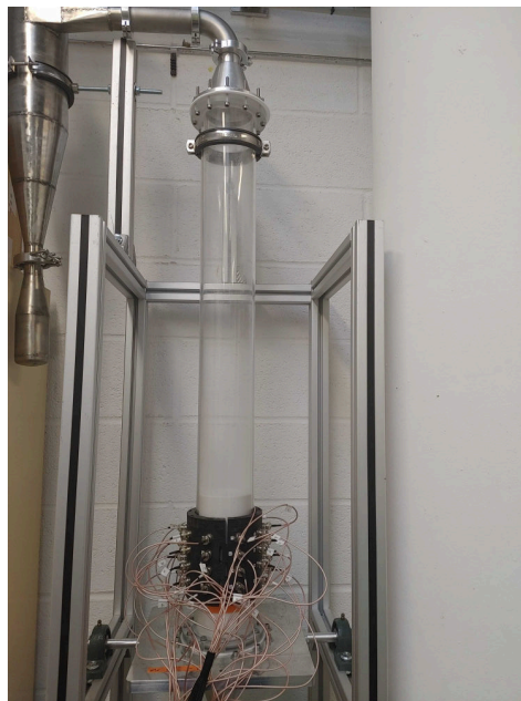
Figure 4.1: Laboratory scale fluidized bed column used with the acquired ECVT device.
