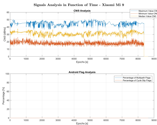
Figure C.5: Signal Analysis of the Xiaomi Mi9. a) Upper Figure: C/N0 Analysis. b) Lower Figure: Percentage of Android Flags Activation
