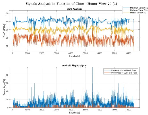
Figure C.3: Signal Analysis of the Honor View 20 (1). a) Upper Figure: C/N0 Analysis. b) Lower Figure: Percentage of Android Flags Activation
