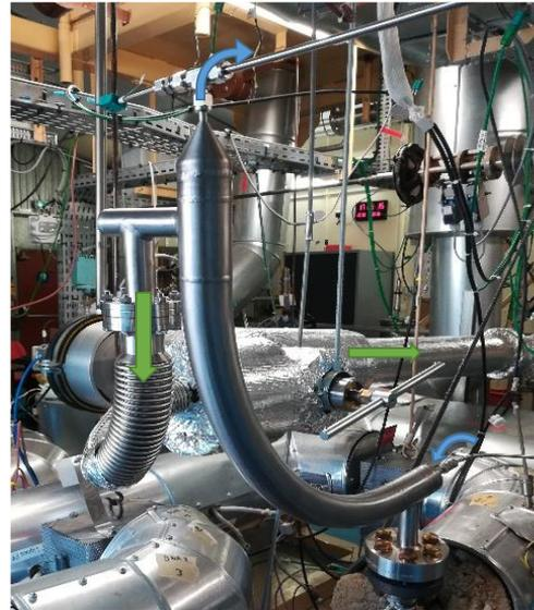
Figure 3-15 Test section installed for gas-vacuum test: details of gas supply system (blue) and UHV (green) connections
