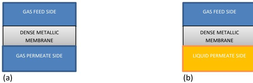
Figure 2-1. Permeation across different domains: gas-metal-gas (a) and gas-metal-liquid (b)
