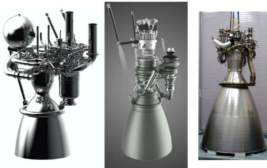
Figure 1.5: Some methane-fed rocket engines. From left to right: Prometheus (ESA/CNES), Raptor (SpaceX), LNG (JAXA). Not at scale.
