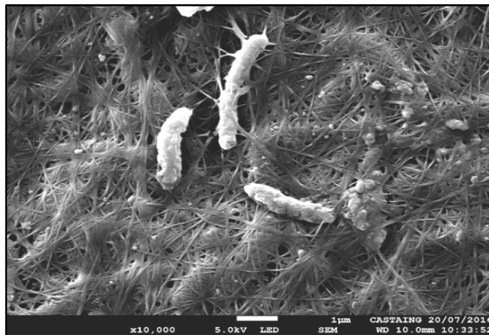
Figure 14. Scanning electron micrograph of bacteria embedded within the cellulose microfibrils from Kombucha tea.
