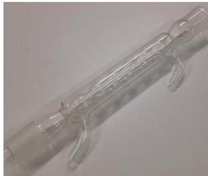
Figure I-24 Colonne de distillation
