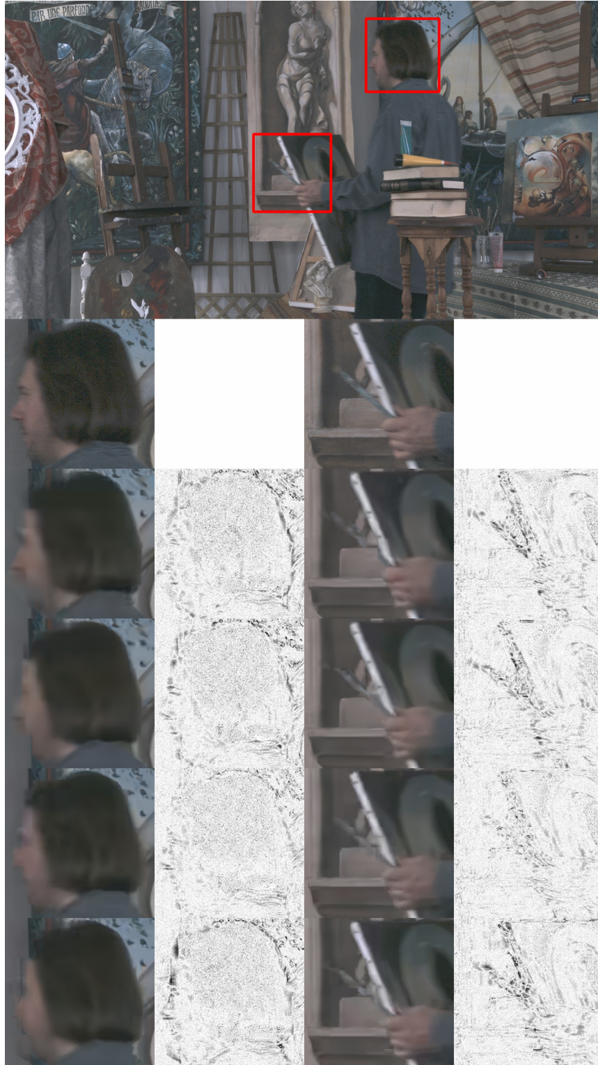
FIGURE 4.1: Details from the compressed texture atlases of the Painter sequence, matching bitrate, all tested encoders. The first row shows the uncompressed source texture. Second row: cropped source, third row: VVenC, fourth row: VTM12, fifth row: AV1, last row: HPM12. The second and fourth columns represent the difference between the encoded atlas and the source.
