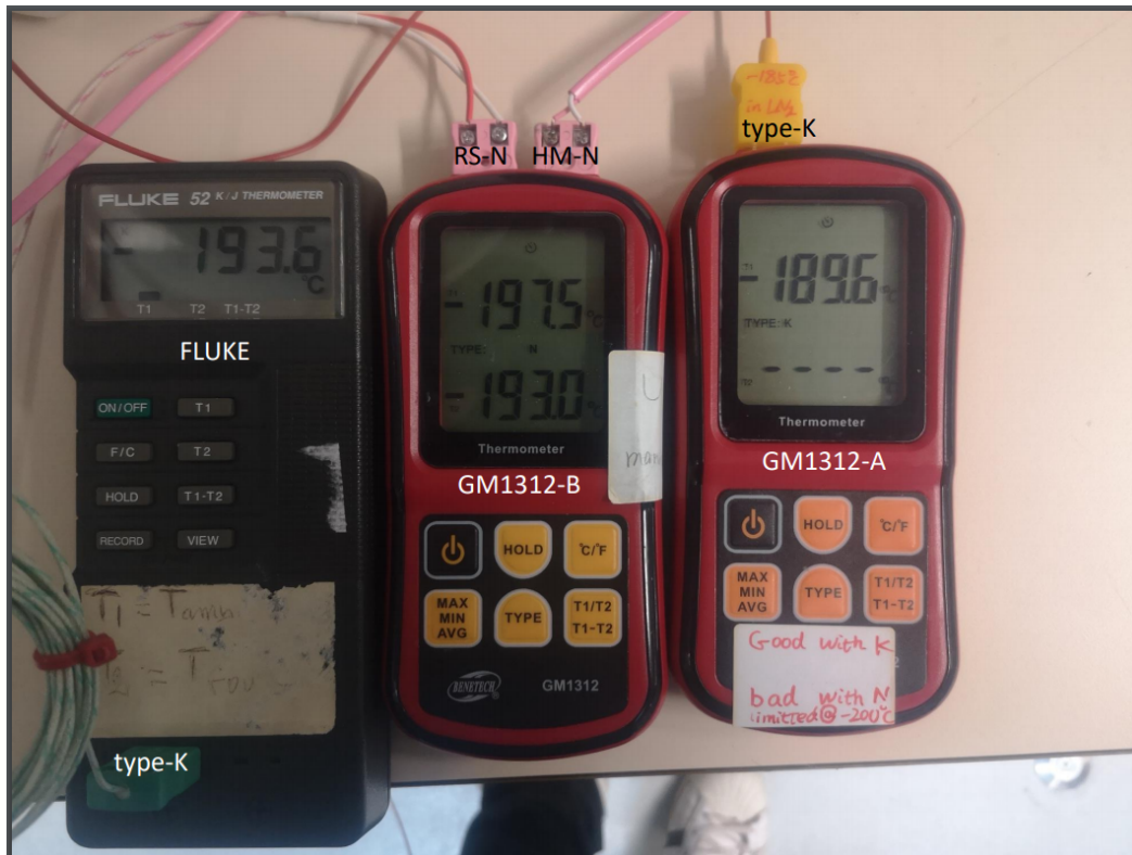
Figure E.2 The temperature was measured by a type-N plug with GM1312B N mode (GM1312B-N), a type-N plug with GM1312B K mode (GM1312B-K), in addition, A type-K plug with Fluke as the reference temperature.
