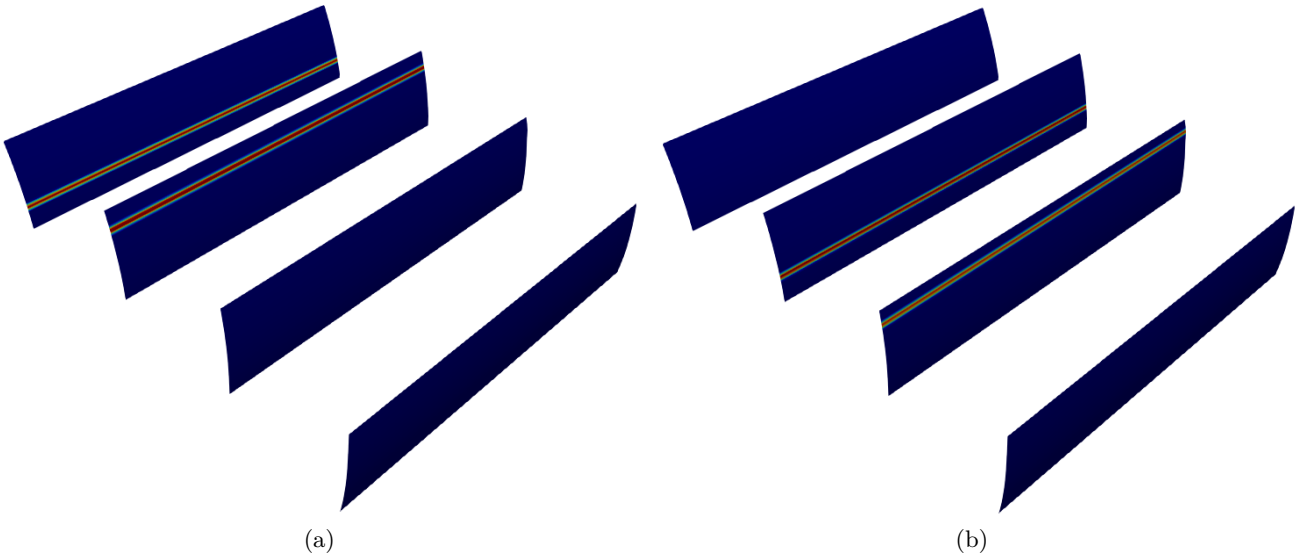
Figure V.15: Example of the field of contact forces for a given position of the driving gear (a) and another position (b)
