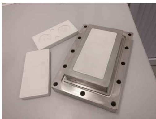
Figure 2.6: metallic holder with the gypsum samples molded in 3D printed cast.
