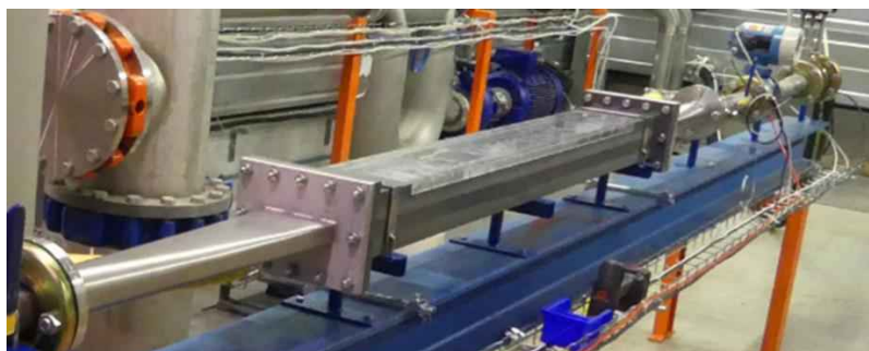
Figure 2.5: view of the rectangular test section. The flow goes from right to left.
