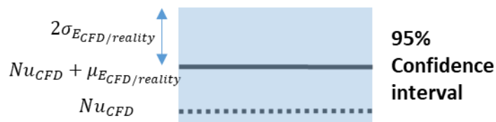
Figure 1.3– calculation of a 95% confidence interval from the computed Nusselt number Nu_{CFD} and the error between CFD and reality E_{CFD/reality}
