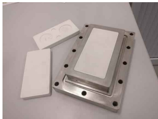
Figure 2.6: metallic holder with the gypsum samples molded in 3D printed cast.
