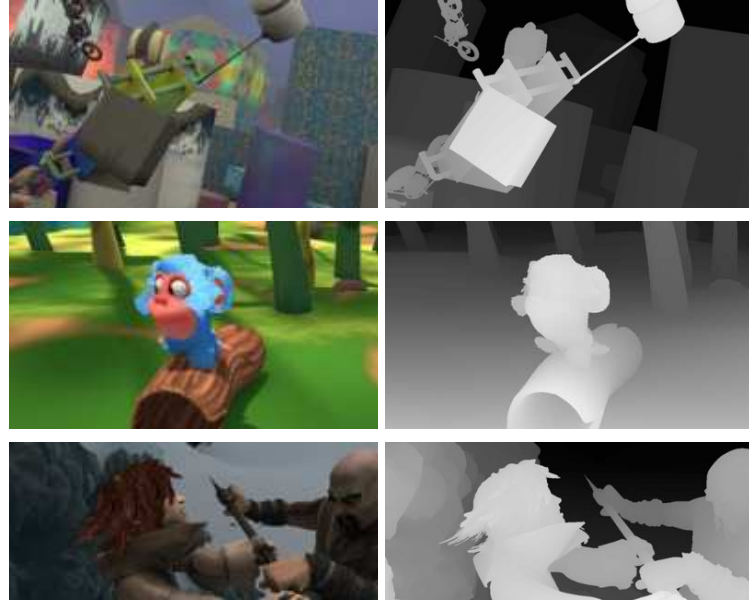
FIGURE 3.1: Examples from the Scene Flow dataset [144, Fig. 7]. This figure illustrates the diversity of this dataset. From left to right are the left color synthetic image and the corresponding disparity map, respectively.
