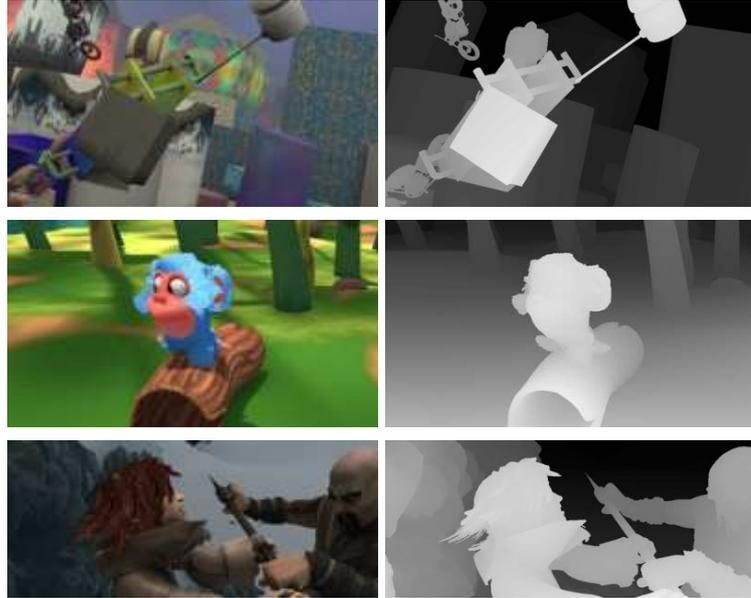
FIGURE 3.1: **Examples from the Scene Flow dataset [144, Fig. 7].** This figure illustrates the diversity of this dataset. From left to right are the left color synthetic image and the corresponding disparity map, respectively.
