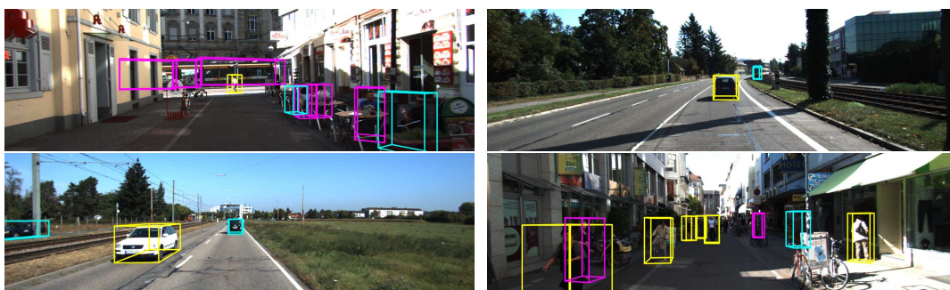
FIGURE 3.6: Example of the difficulty level of the objects in the KITTI dataset corresponding to the definition in Table 3.3. Easy, Moderate and Hard objects are shown in yellow, blue and pink 3D bounding boxes.
