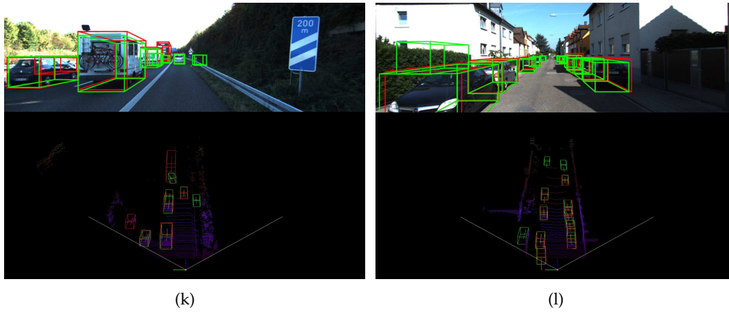
FIGURE 4.9: Qualitative Comparison. We illustrate the results of SLS-Fusion with different input point clouds on a KITTI validation scene. They are visualized in a frontal-view image as well as a BEV point map. Ground-truth and predicted boxes are in red and green, respectively.
