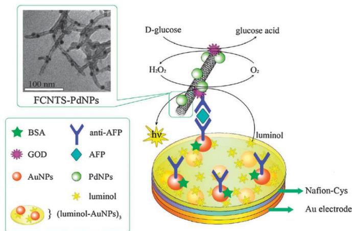
Figure 16. Representation of ECL-based sandwich-type immunosensor and the synergetic catalysis effect of GOD and PdNPs for ultrasensitive immunoassay of AFP.<sup>120</sup>
