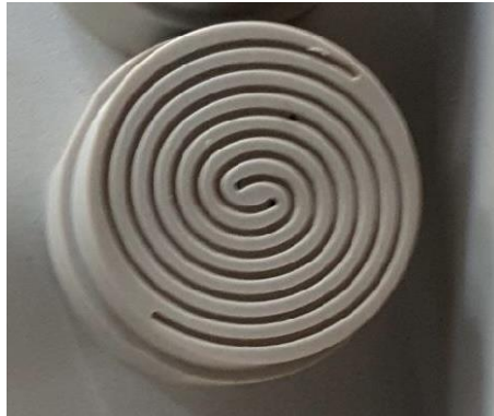
Figure 123 - Double-spiral diffuser used for HDT experiments of Estailades limestone samples.
