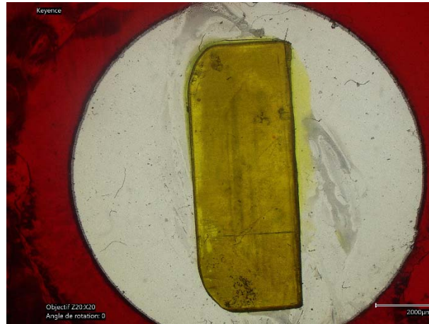
Fig. 4.7 Image of the 0.38 mm thick single BNA crystal fabricated by Swiss THz technology, which was used in this work. It has a damage threshold of 3.7 \text{ mJ/cm}^2 .
