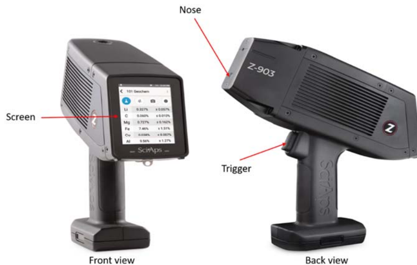
Fig. 5.20 Front and back view of the SciAps Z-903 handheld laser-induced breakdown spectroscopy analyzer.
