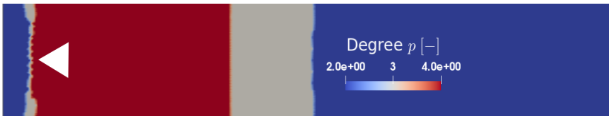
Figure 8.27. – Polynomial degree distribution near the bluff-body region for the reacting case in the xy -plane.
