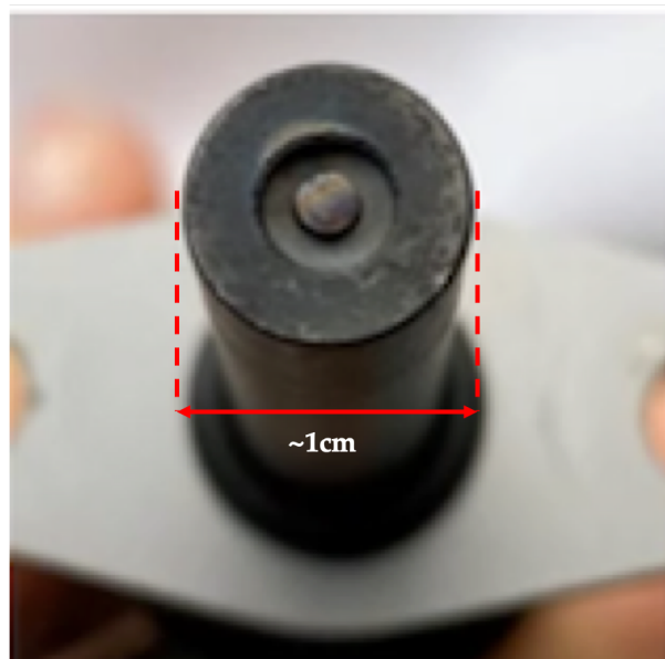
Figure 0.2.2: Illustration of an aeronautical spark plug ignition system
