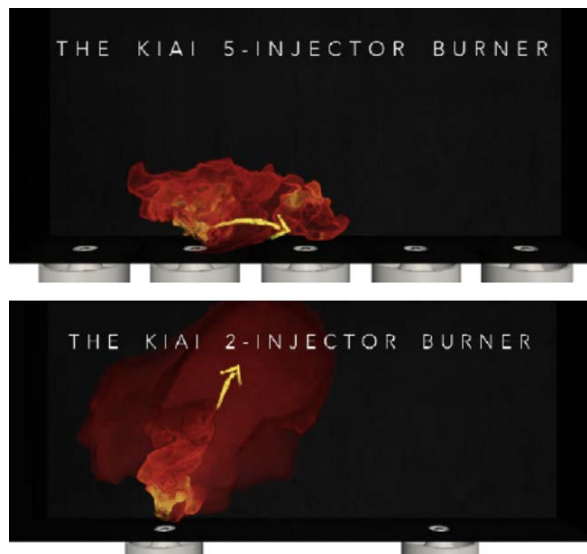
Figure 2-17: Above: spanwise mode of propagation for low inter-burner space. Below "arc" mode for high inter-burner space [18]
