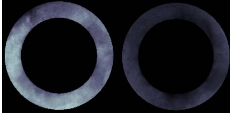
Figure 8-39: (Left) Direct visualization image for case \alpha = 23^\circ and \phi = 0.7 . (Right) Direct visualization image for case \alpha = 0^\circ and \phi = 0.7 . Both images taken at the instant of maximum luminosity, the weaker luminosity in the case \alpha = 0^\circ indicates weaker chemical activity (Courtesy of Yi-Hao Kwah (NTNU))
