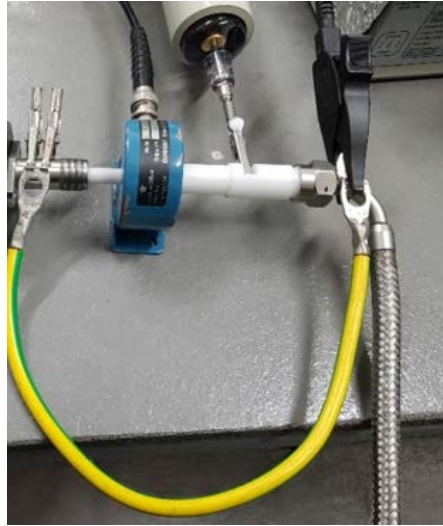
Figure 6-2: Adaptation to measure temporal current and voltage evolution
