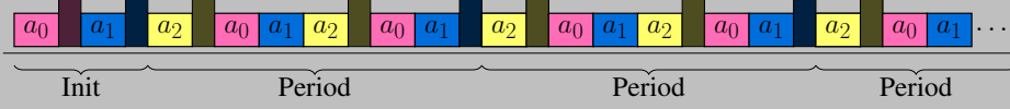
Figure 2.3: A periodic schedule represented graphically for a job where each iteration consists of three tasks a_0, a_1, a_2 [J2].
