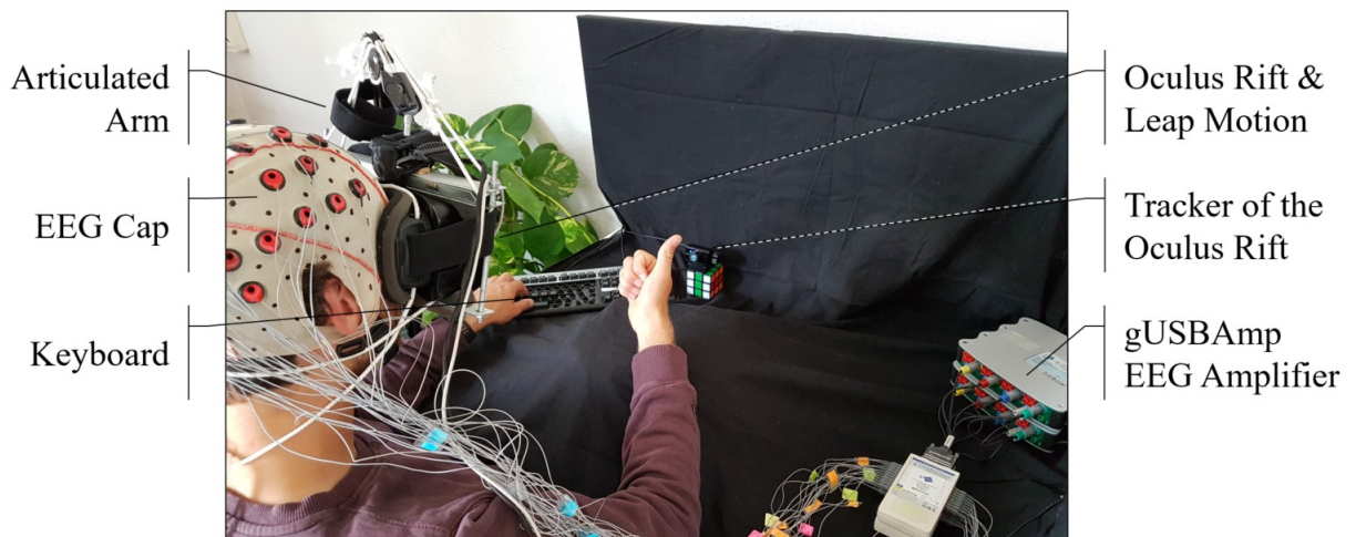
Figure 3.2 – Experimental setup used in Jeunet et al. [Jeu+18]. Participants wore an EEG headset and were immersed in a virtual environment with an Oculus Rift attached to an articulated arm. Participant’s right hand was tracked by a Leap Motion fixed on top on the Oculus Rift. Figure from Jeunet et al.
