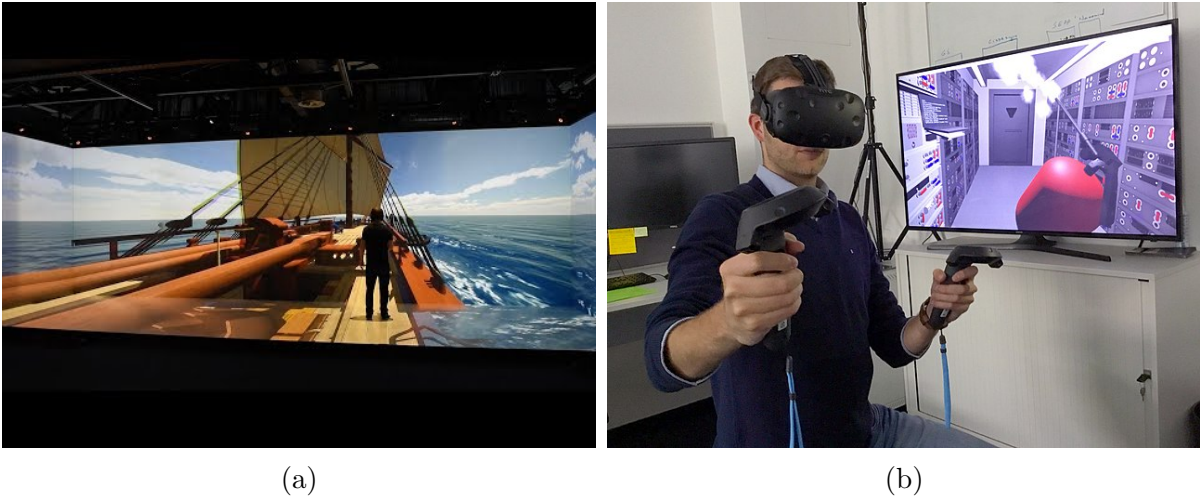
Figure 2 – (a) Example of a CAVE named Immersia located in Rennes, France. (b) Example of a HMD use case. The user is an astronaut training in VR to to extinguish a fire inside a lunar habitat. By ESA, CC BY-SA IGO 3.0.
